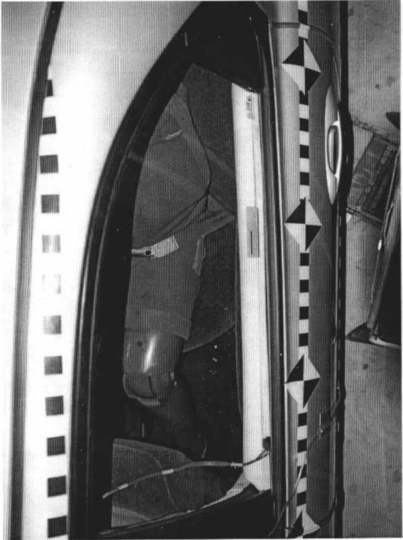
Figure A-30: Passenger Dummy Clearance, Pre-Test
