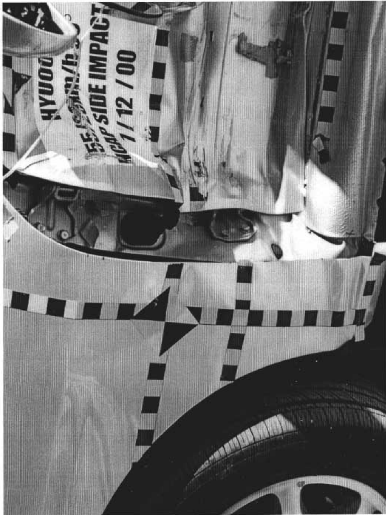
Figure A-17: Impact Point Target Close-up, Post-Test
