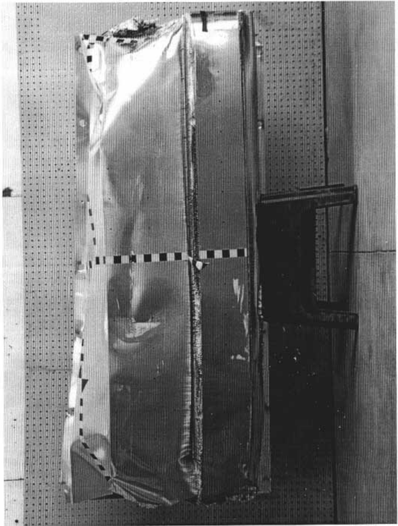
Figure A-37: Front View of Deformable Barrier, Post-Test
