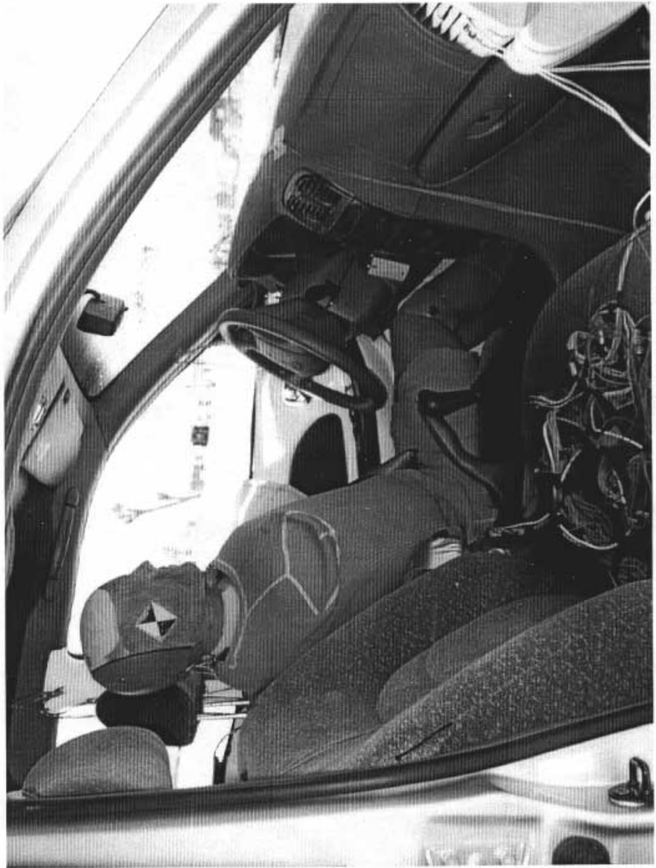
Figure A-24: Driver Dummy Inside View, Post-Test
