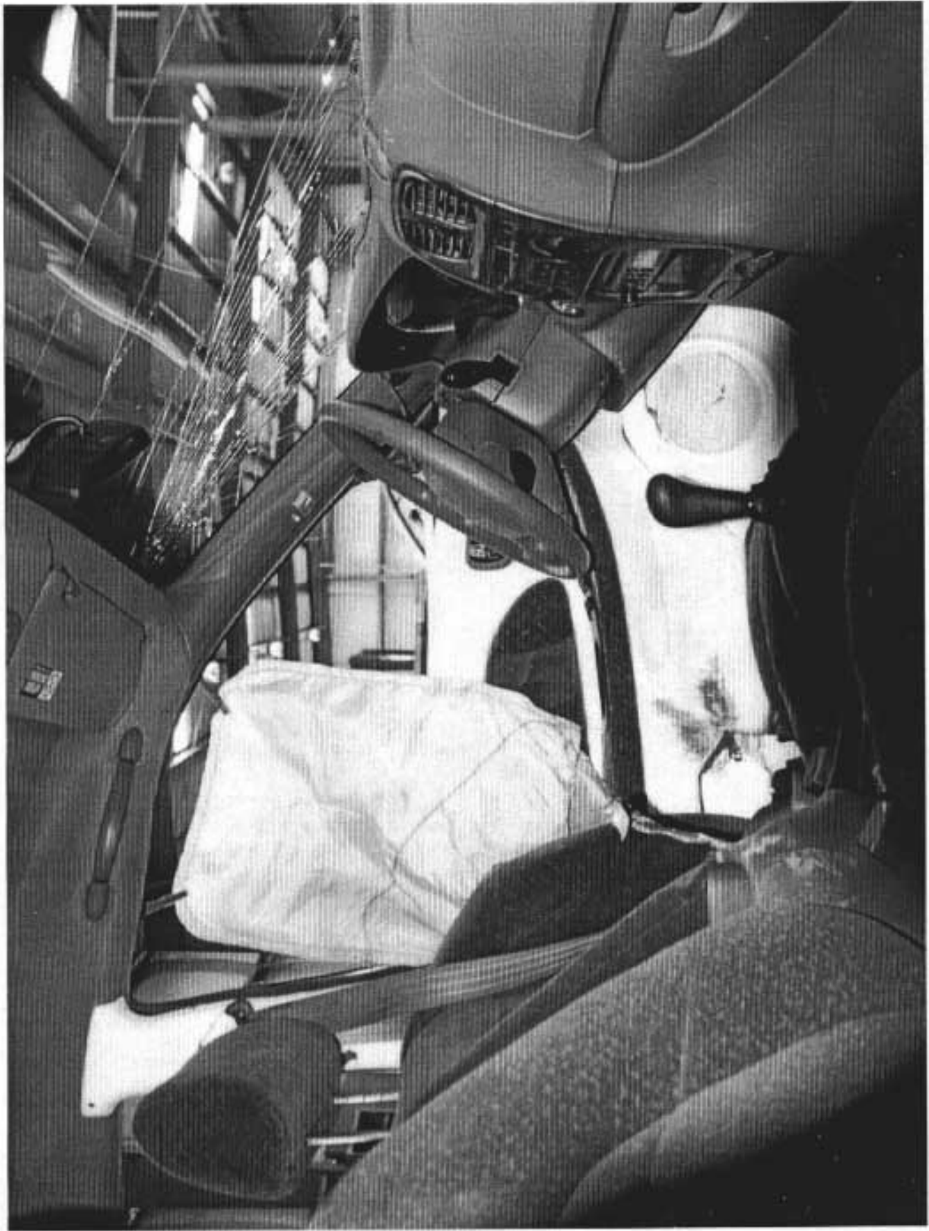
Figure A-26: Driver Dummy Contact Points Inside View, Post-Test
