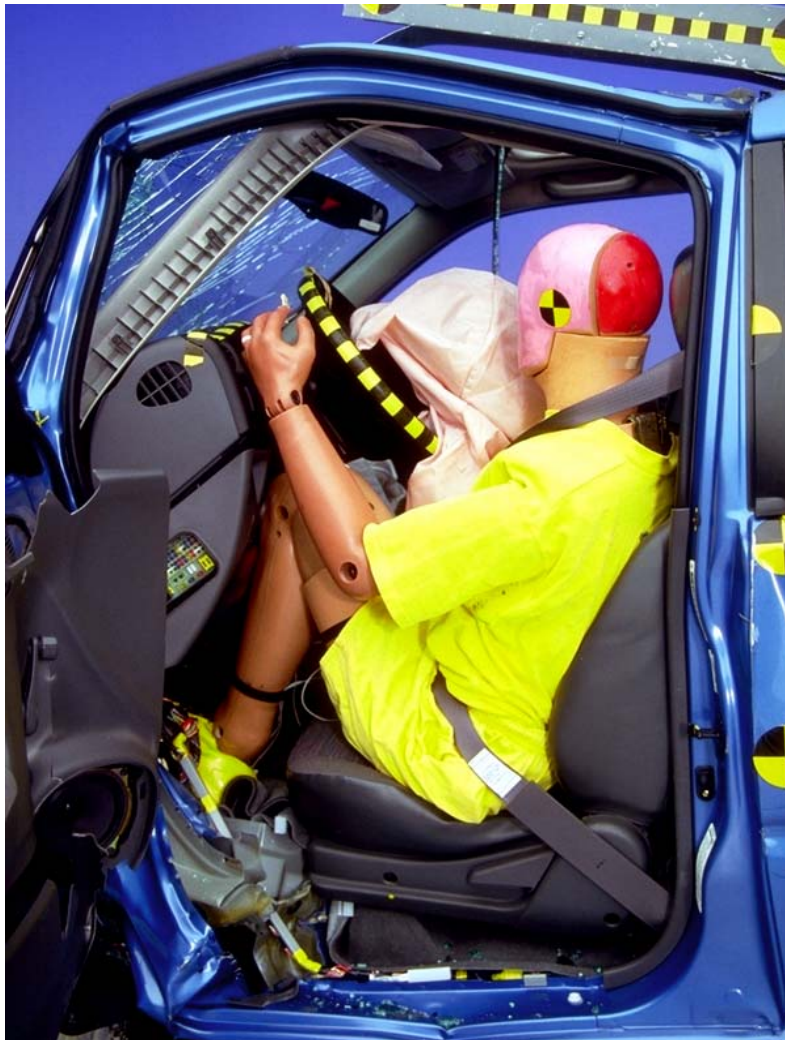
Figure 7 Dummy and Vehicle Interior, Postcrash — 1998 Isuzu Amigo
