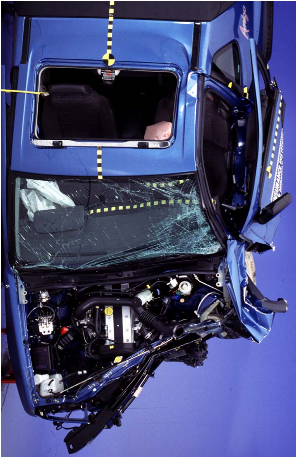
Figure 2 Overhead View of Crash Deformation — 1998 Isuzu Amigo
