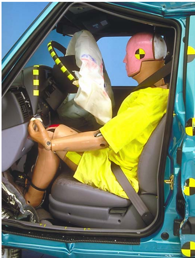
Figure 7 Dummy and Vehicle Interior, Postcrash — 1998 Jeep Cherokee
