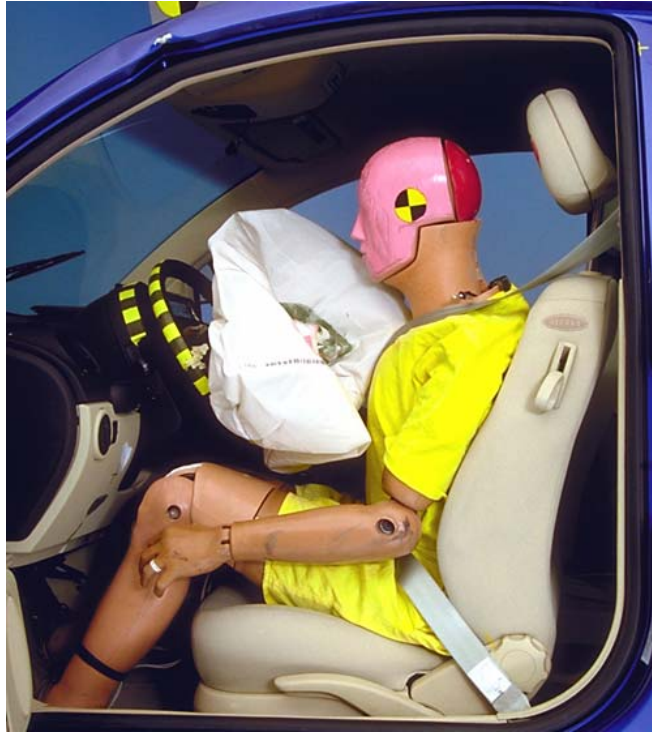
Figure 7 Dummy and Vehicle Interior, Postcrash — 1998 Volkswagen New Beetle
