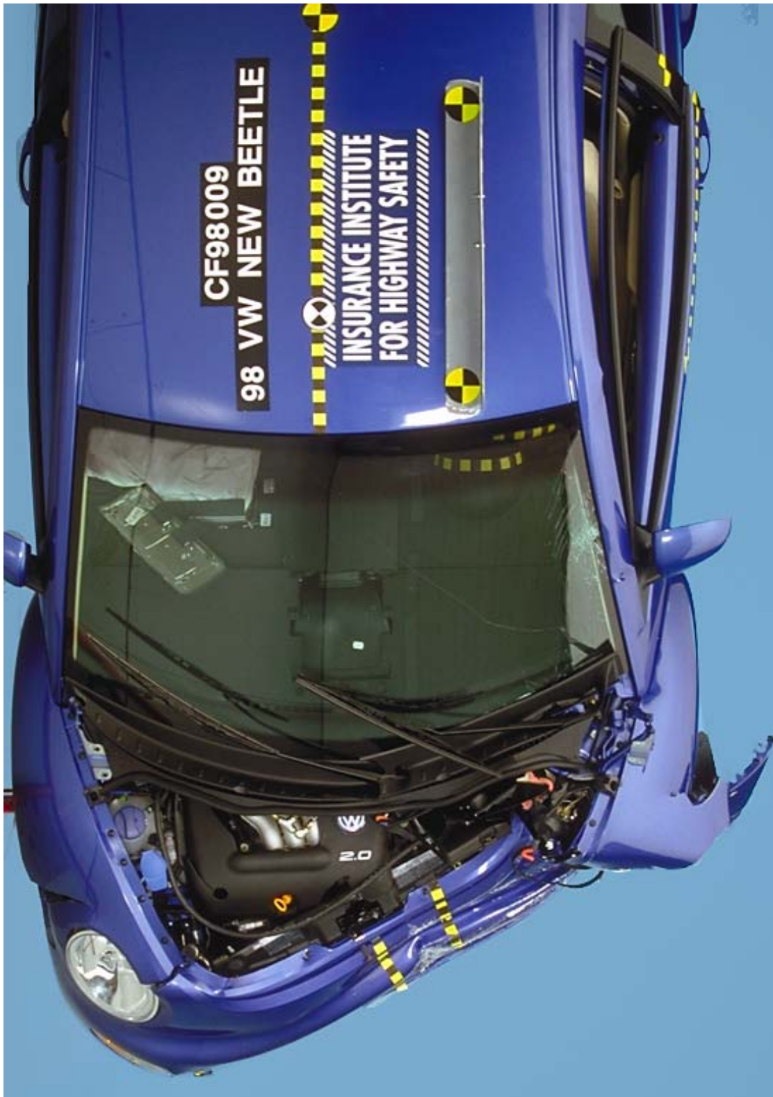
Figure 2 Overhead View of Crash Deformation — 1998 Volkswagen New Beetle
