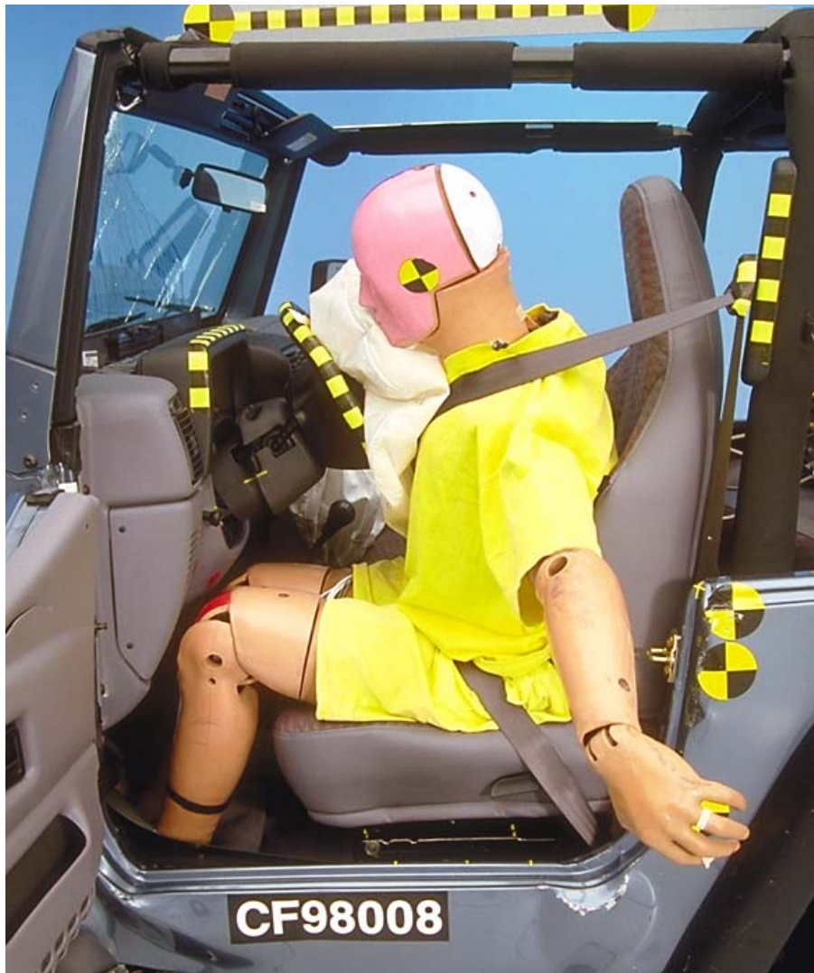
Figure 7 Dummy and Vehicle Interior, Postcrash — 1998 Jeep Wrangler
