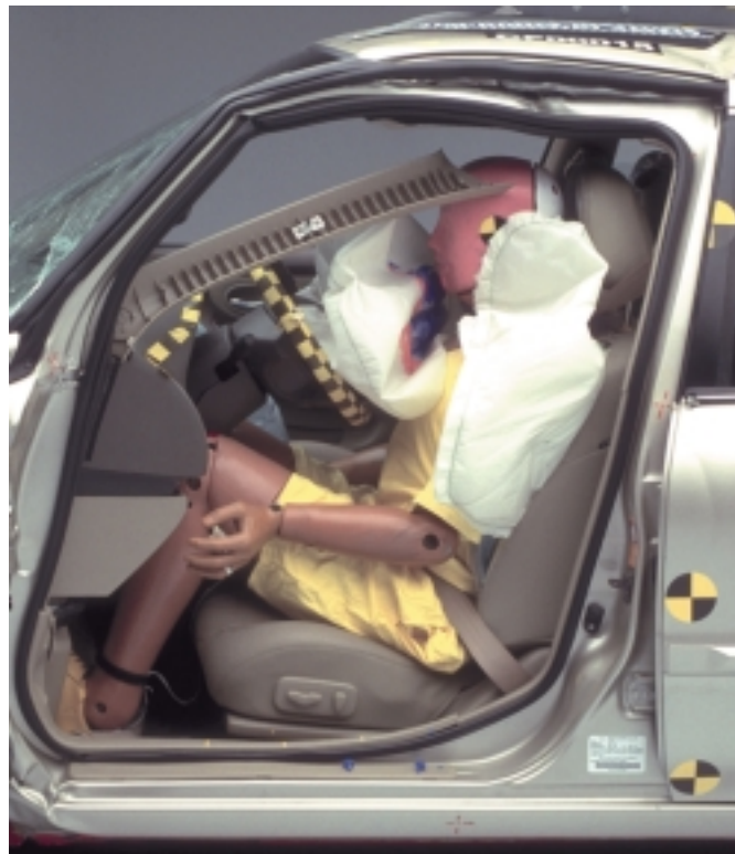
Figure 6 Dummy and Vehicle Interior, Postcrash – 2000 Nissan Maxima
