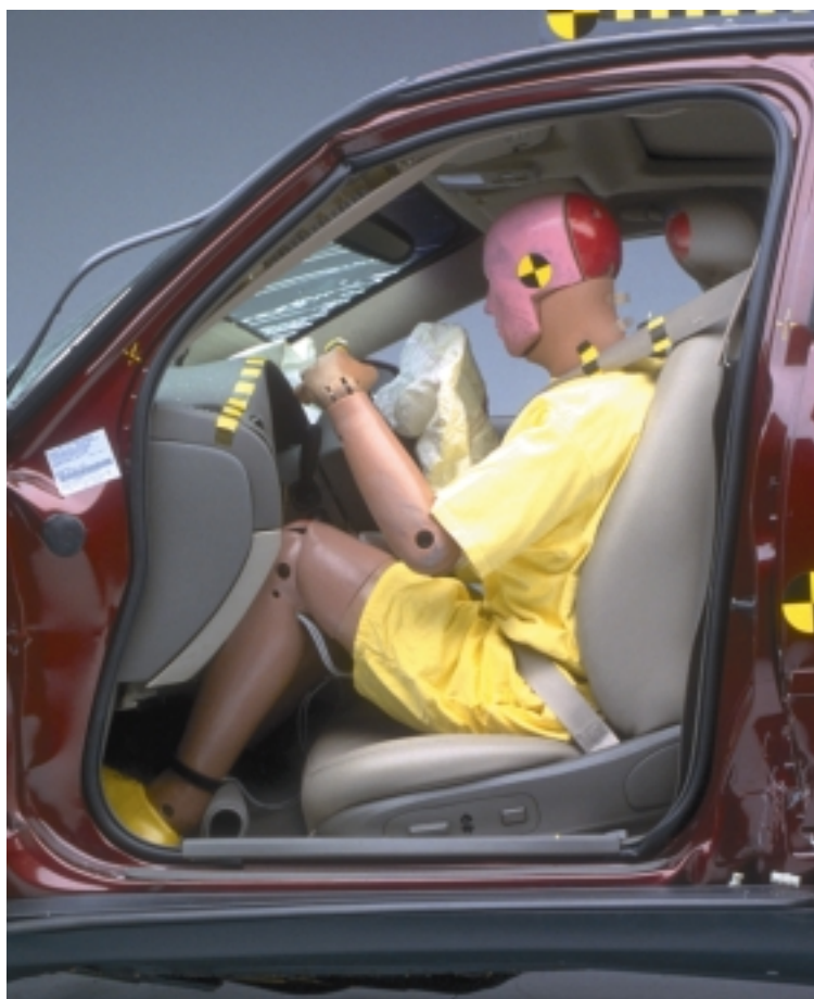
Figure 6 Dummy and Vehicle Interior, Postcrash — 2000 Lincoln LS
