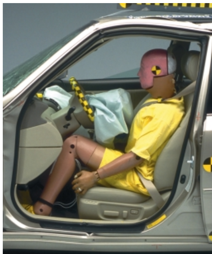
Figure 6 Dummy and Vehicle Interior, Postcrash — 2000 Toyota Avalon
