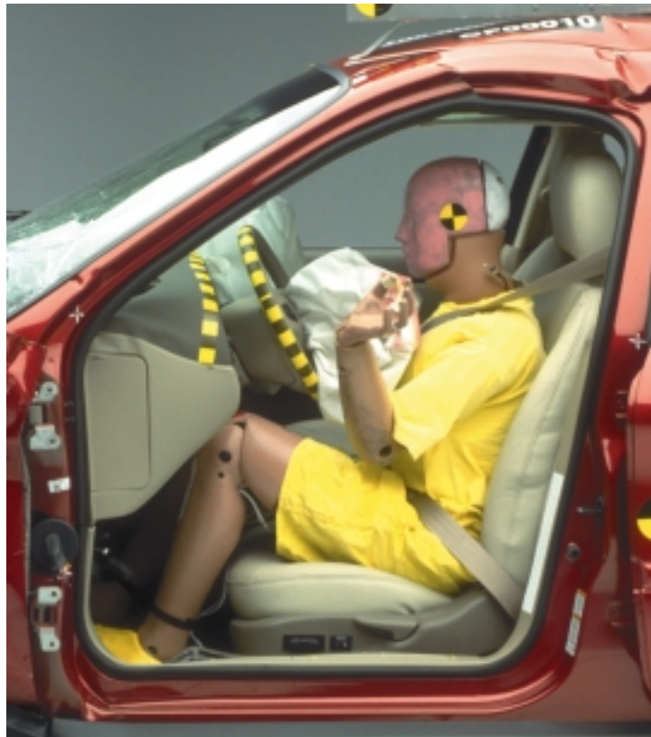
Figure 6 Dummy and Vehicle Interior, Postcrash – 2000 Ford Taurus
