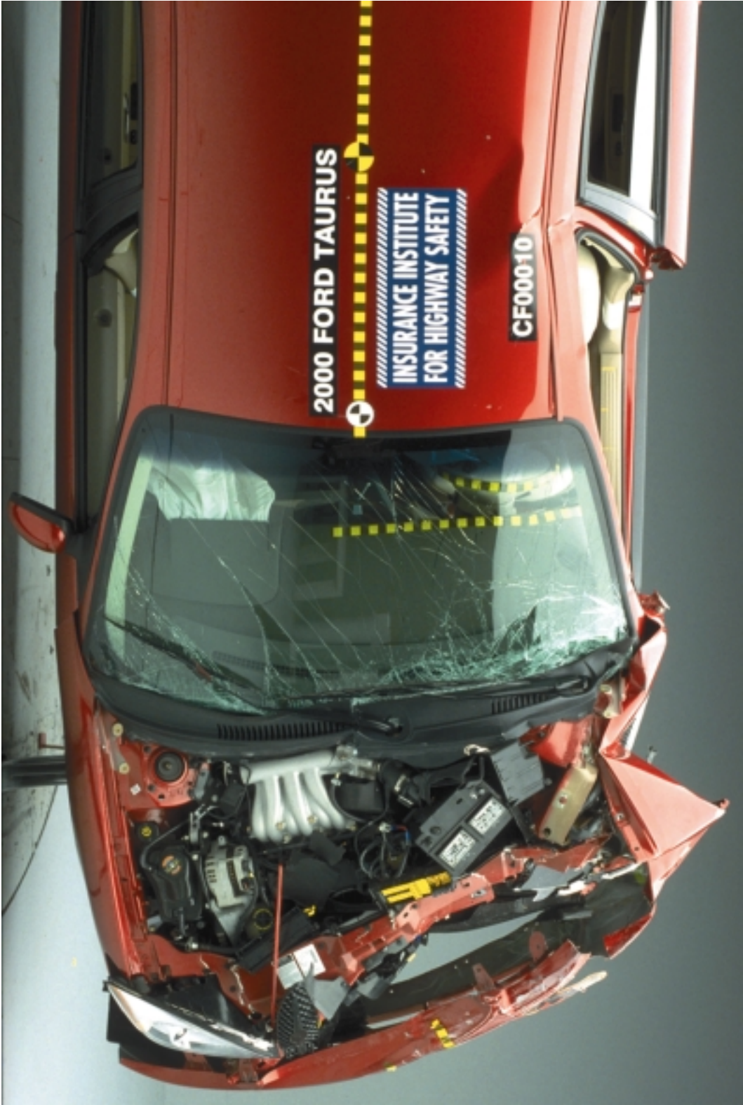
Figure 2 Overhead View of Crash Deformation – 2000 Ford Taurus
