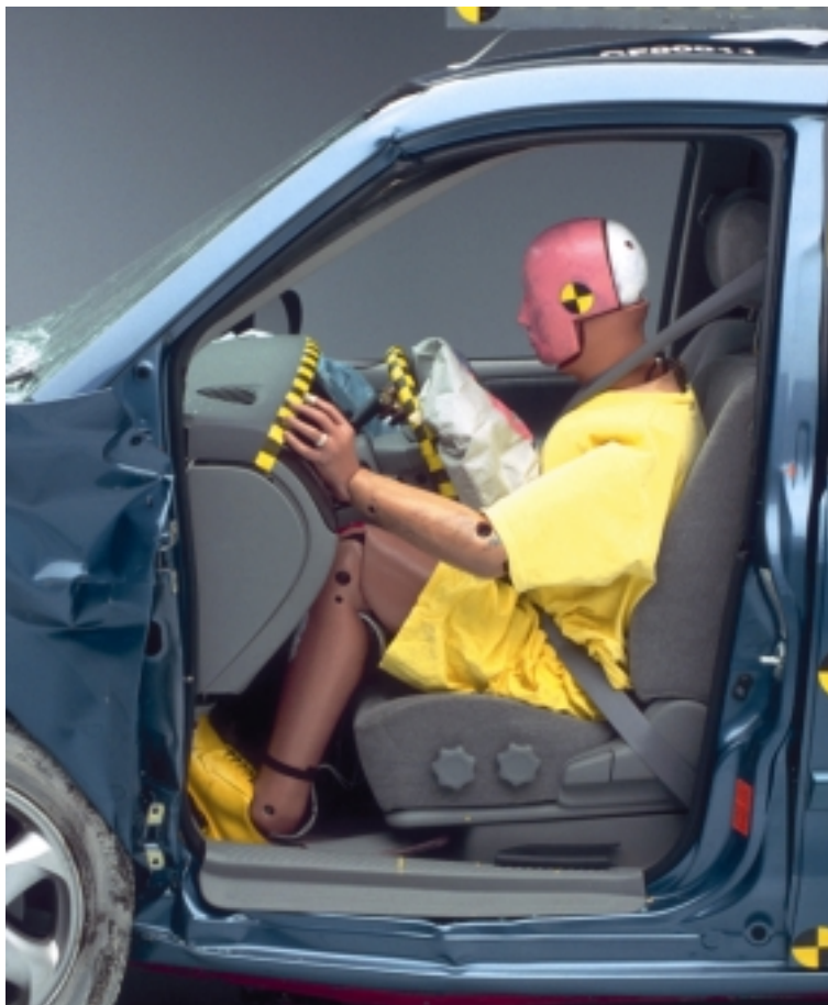
Figure 6 Dummy and Vehicle Interior, Postcrash – 2000 Mazda MPV
