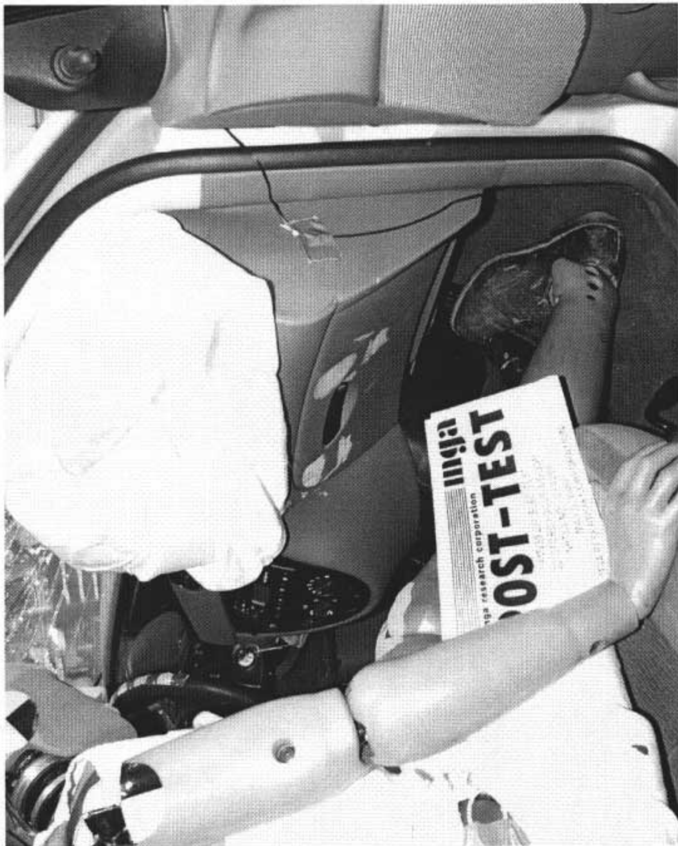
Photo No. A-21 - Post-Test Passenger Knee Bolster View
