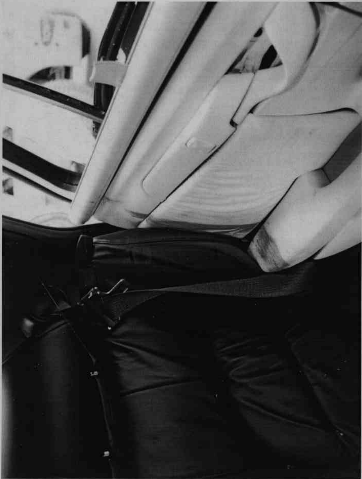
Figure A-46: Rear Seat Side Airbag, Post-Test
