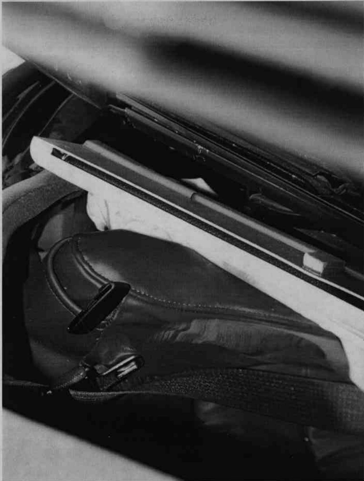
Figure A-47: Rear Seat Side Airbag Close-Up, Post-Test
