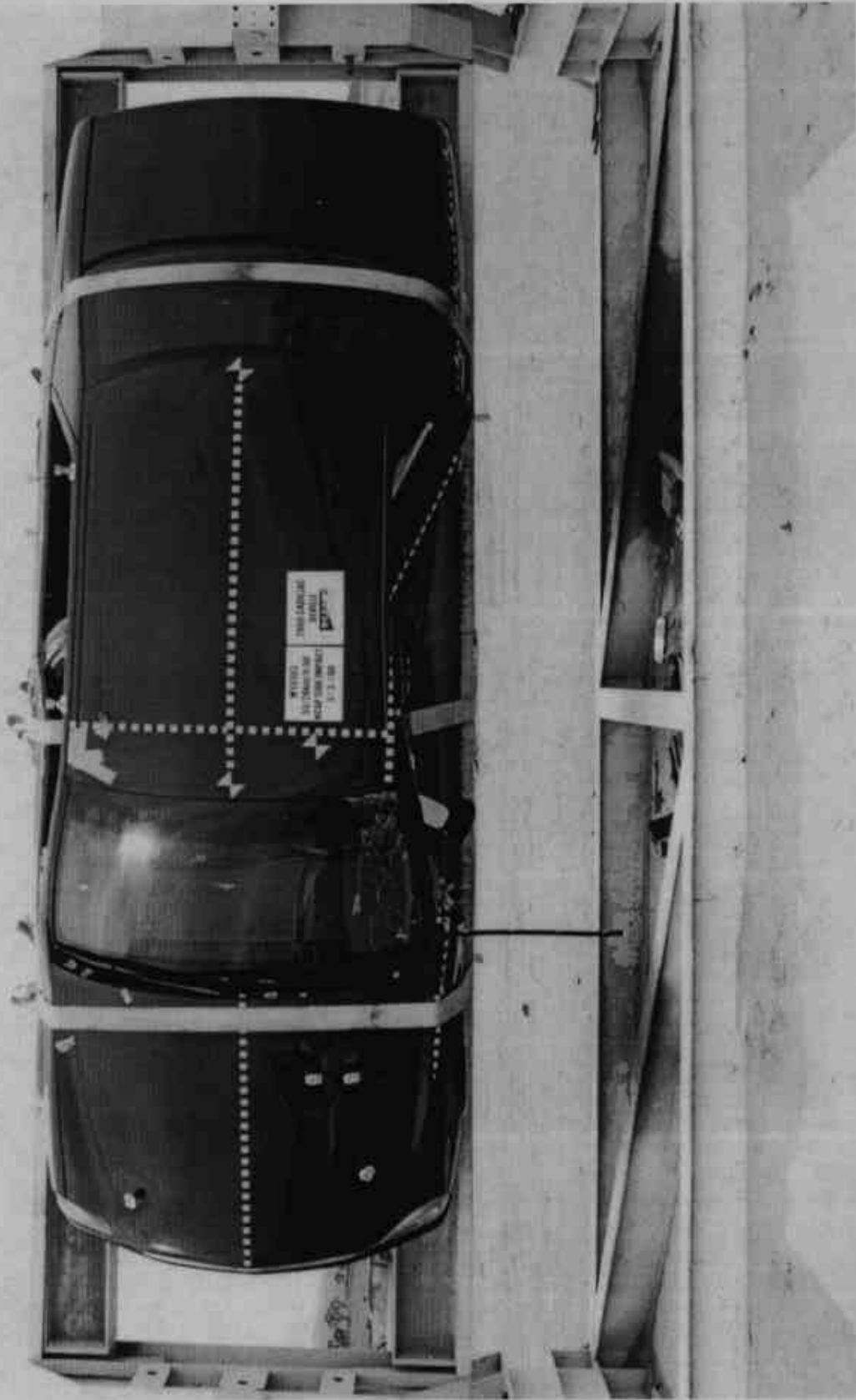
Figure A-44: Vehicle on Rollover Device, Top View
