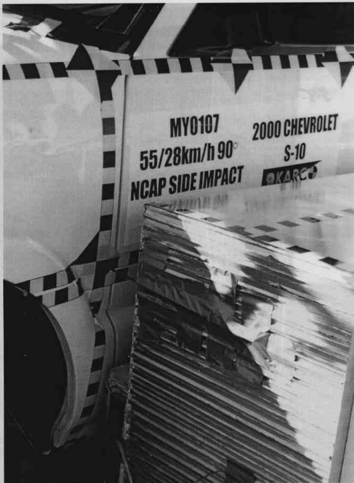
FIGURE A-16: PRE-TEST IMPACT POINT TARGET CLOSE-UP
