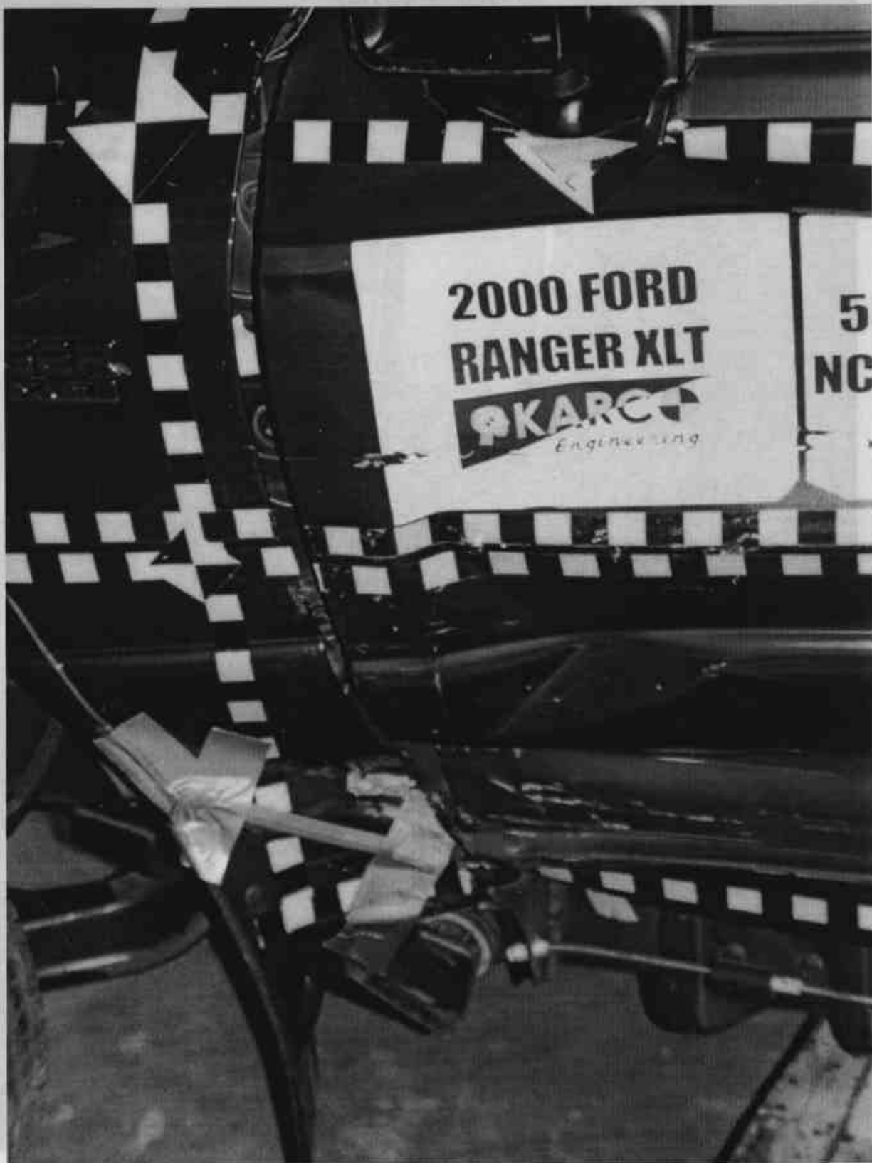
FIGURE A-17: POST-TEST IMPACT POINT TARGET CLOSE-UP
