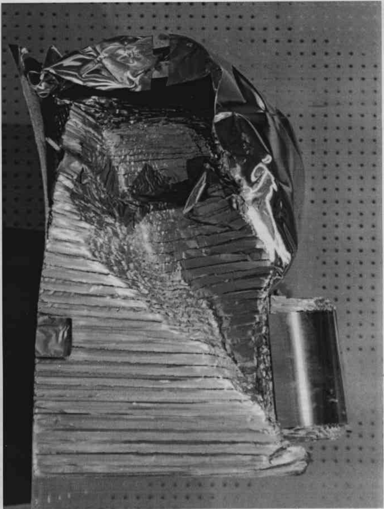
FIGURE A-32: POST-TEST RIGHT SIDE VIEW OF DEFORMABLE BARRIER
