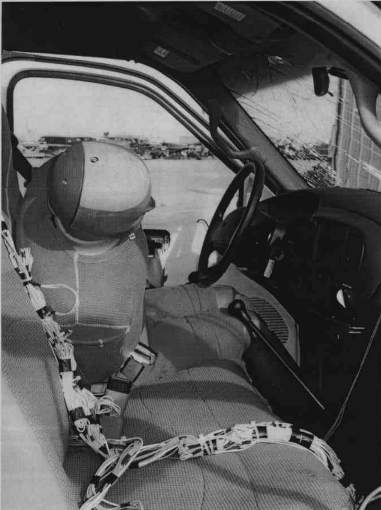
FIGURE A-24: POST-TEST DRIVER DUMMY INSIDE VIEW
