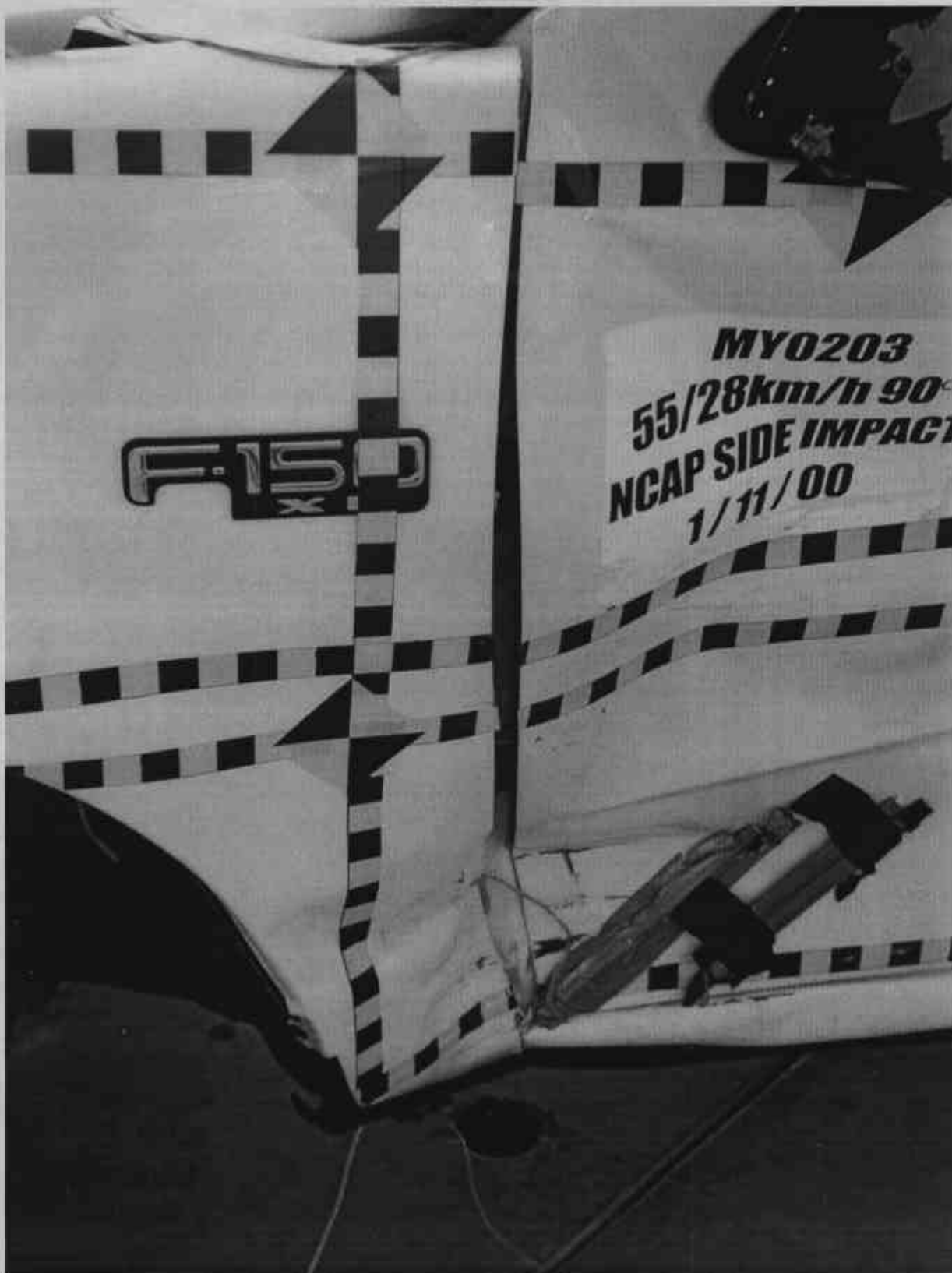
FIGURE A-17: POST-TEST IMPACT POINT TARGET CLOSE-UP
