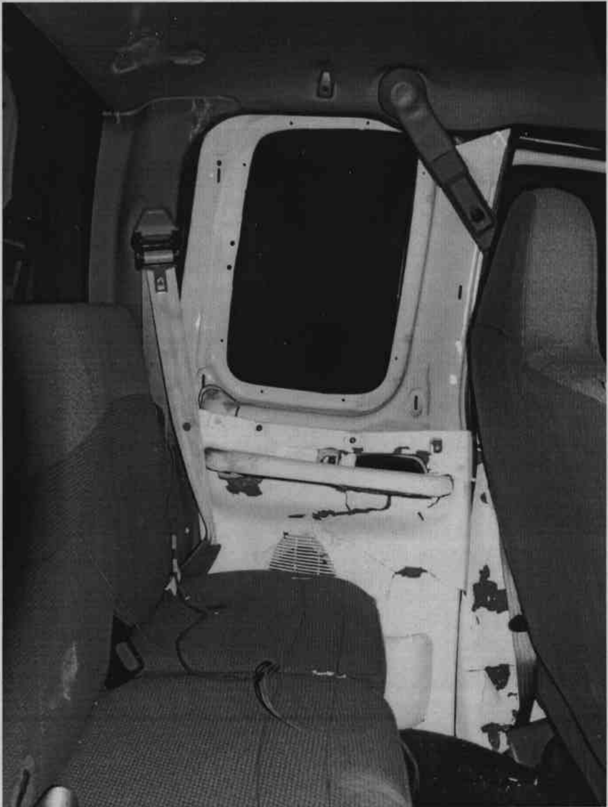
FIGURE A-35: POST-TEST PASSENGER DUMMY CONTACT POINTS (INSIDE VIEW)
