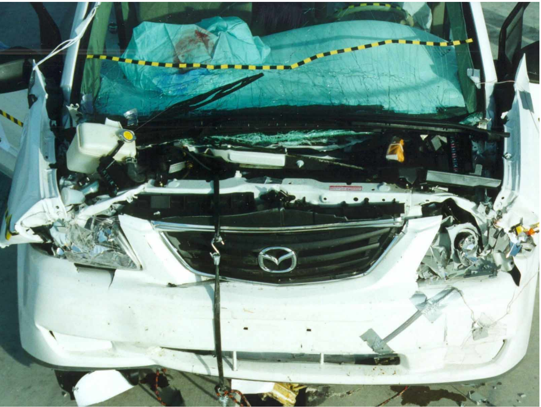
FIGURE A-18. POST TEST ENGINE COMPARTMENT
