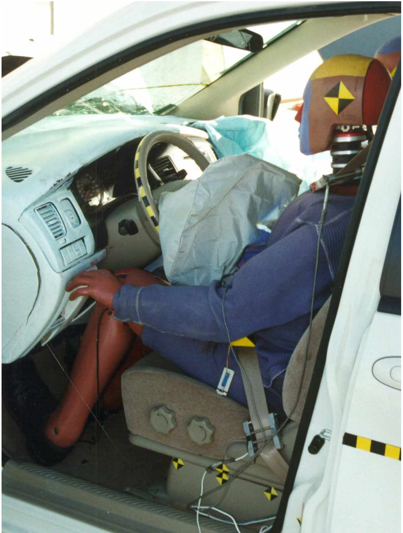
FIGURE A-30. POST TEST DRIVER DUMMY (DOOR OPEN)
