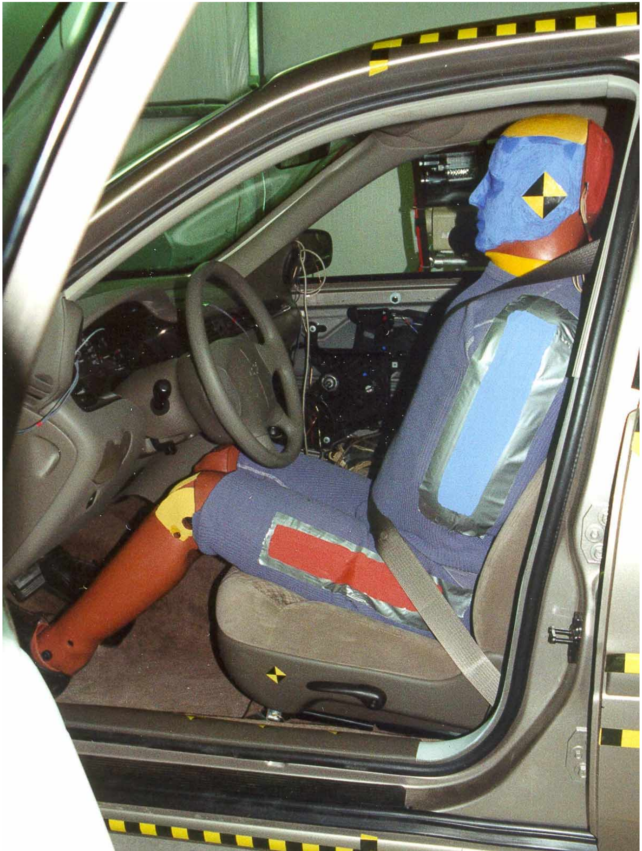
FIGURE A-17: PRE-TEST DRIVER DUMMY LEFT SIDE (DOOR OPEN)
