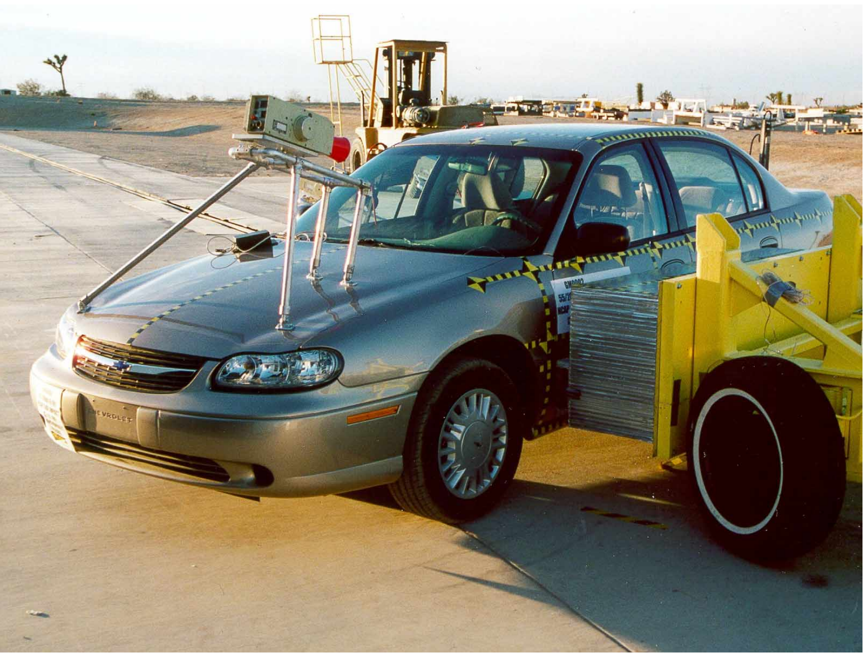
FIGURE A-13: PRE-TEST MDB LEFT SIDE VIEW (AT IMPACT POSITION)
