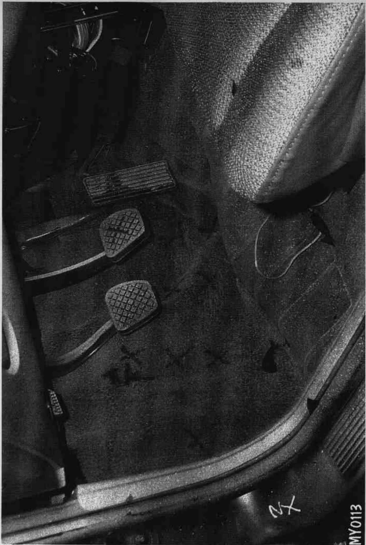
Figure A-35: POST-TEST DRIVER FLOOR PAN VIEW
