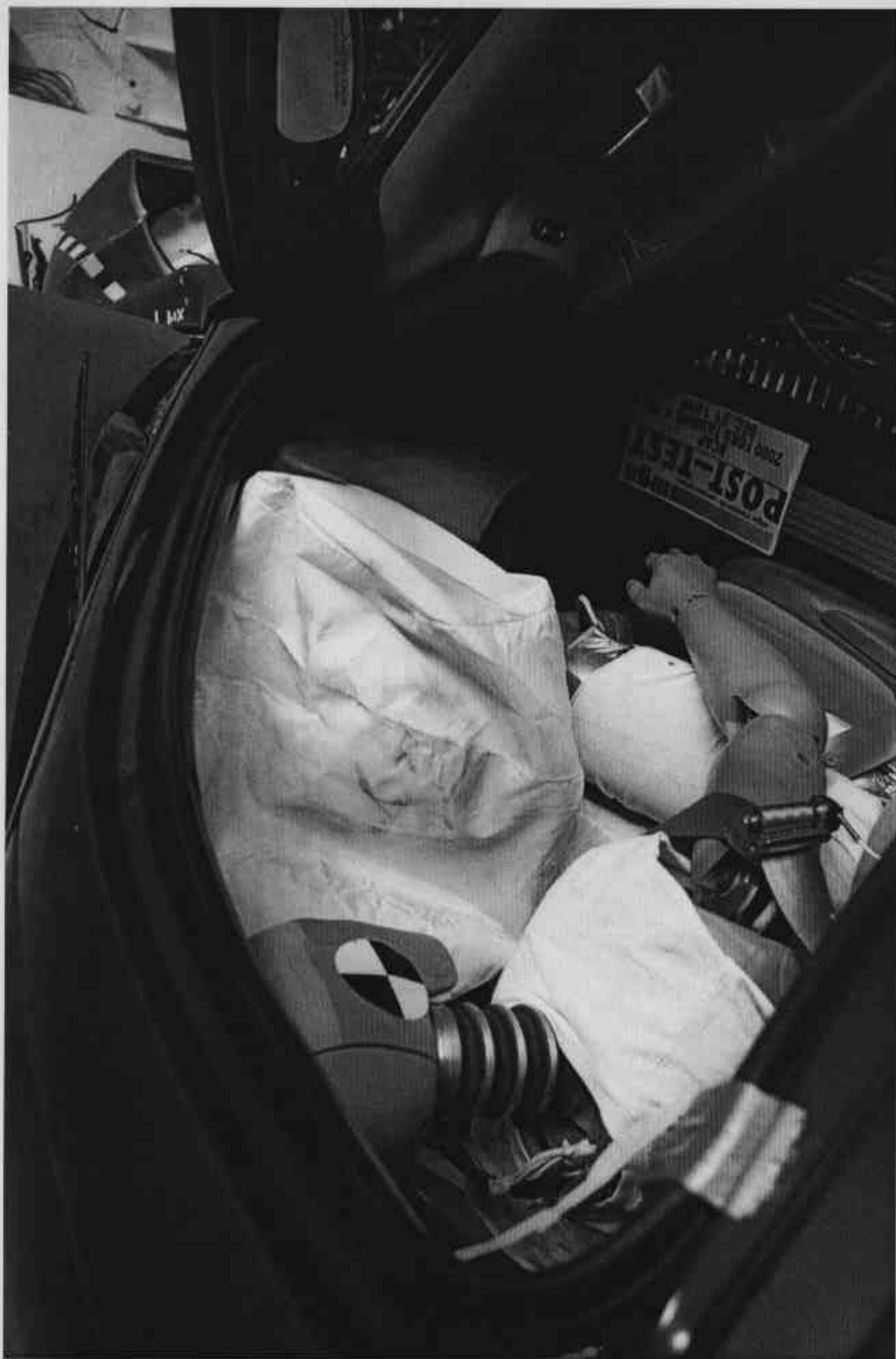
Photo No. A-42 - Post-Test Passenger Airbag Contact
