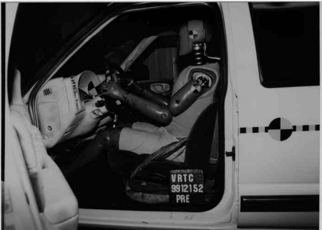
Figure A-32 Pre-Test Driver Dummy Position - View 2
