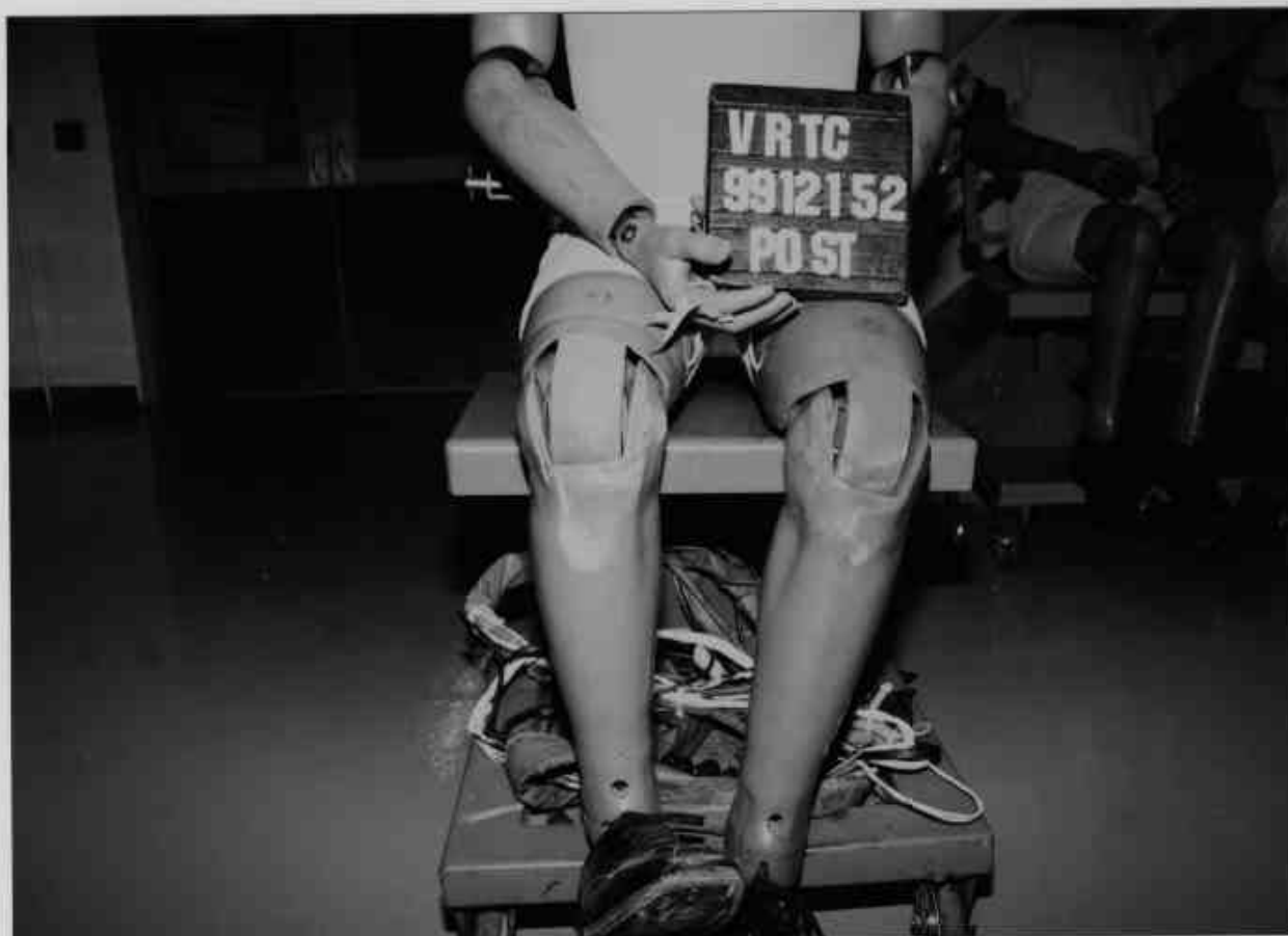
Figure A-45 Post-Test Driver Dummy Knee Contact - View 1
