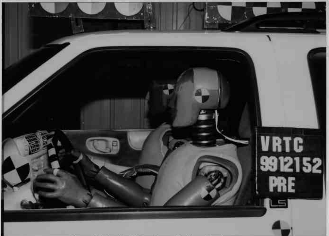
Figure A-30 Pre-Test Driver Dummy Position - View 1
