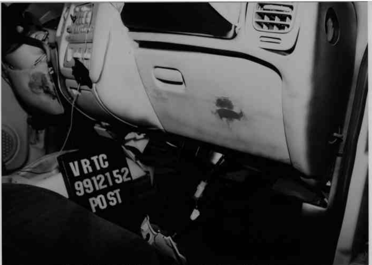
Figure A-52 Post-Test Passenger Dummy Knee Contact - View 2
