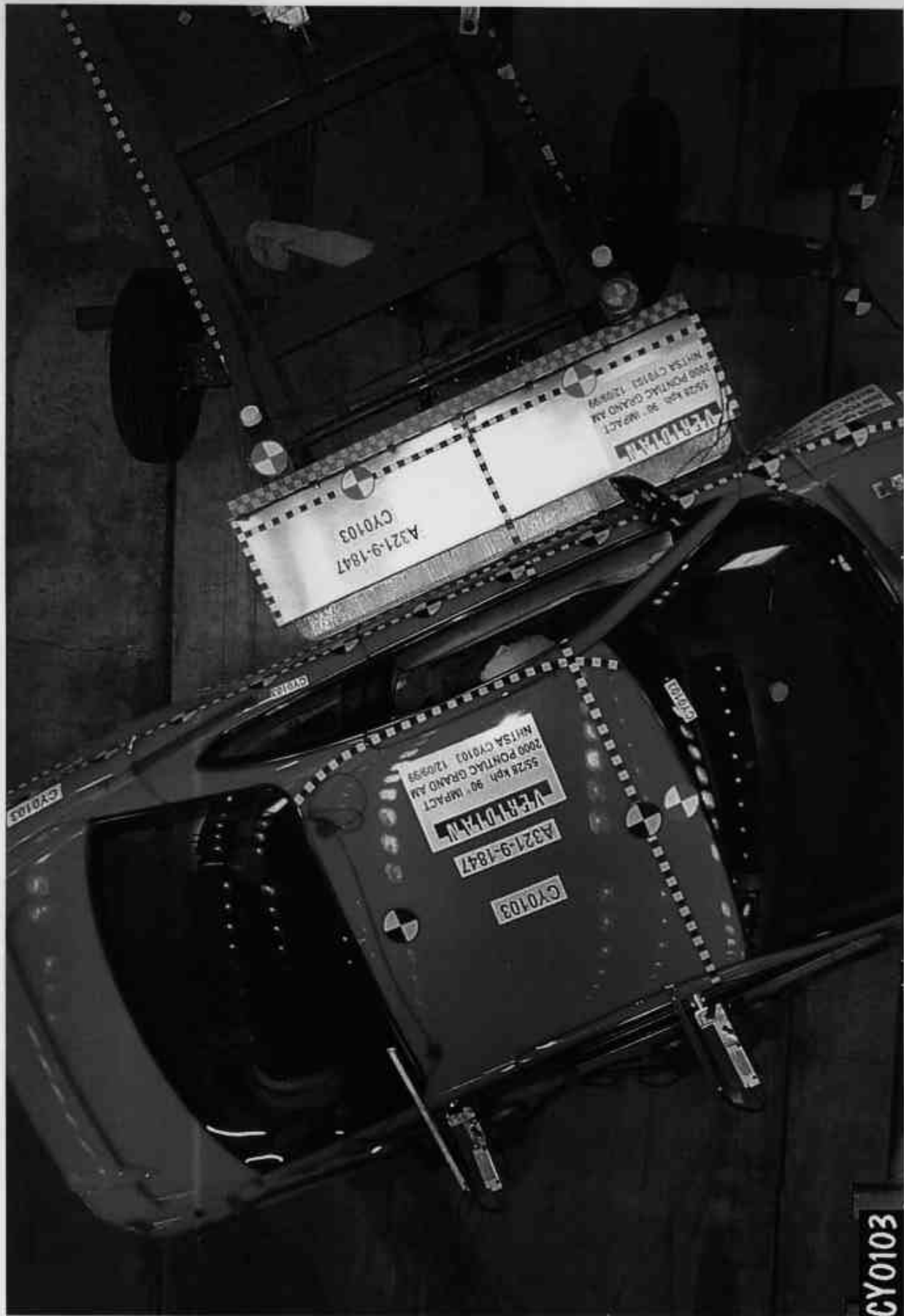
Figure A-15: PRE-TEST OVERHEAD VIEW OF ALIGNED MDB AND VEHICLE
