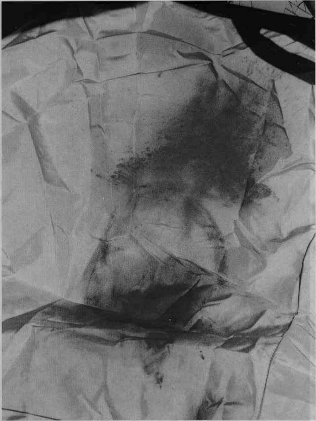
FIGURE A-56. POST TEST PASSENGER DUMMY CONTACT
