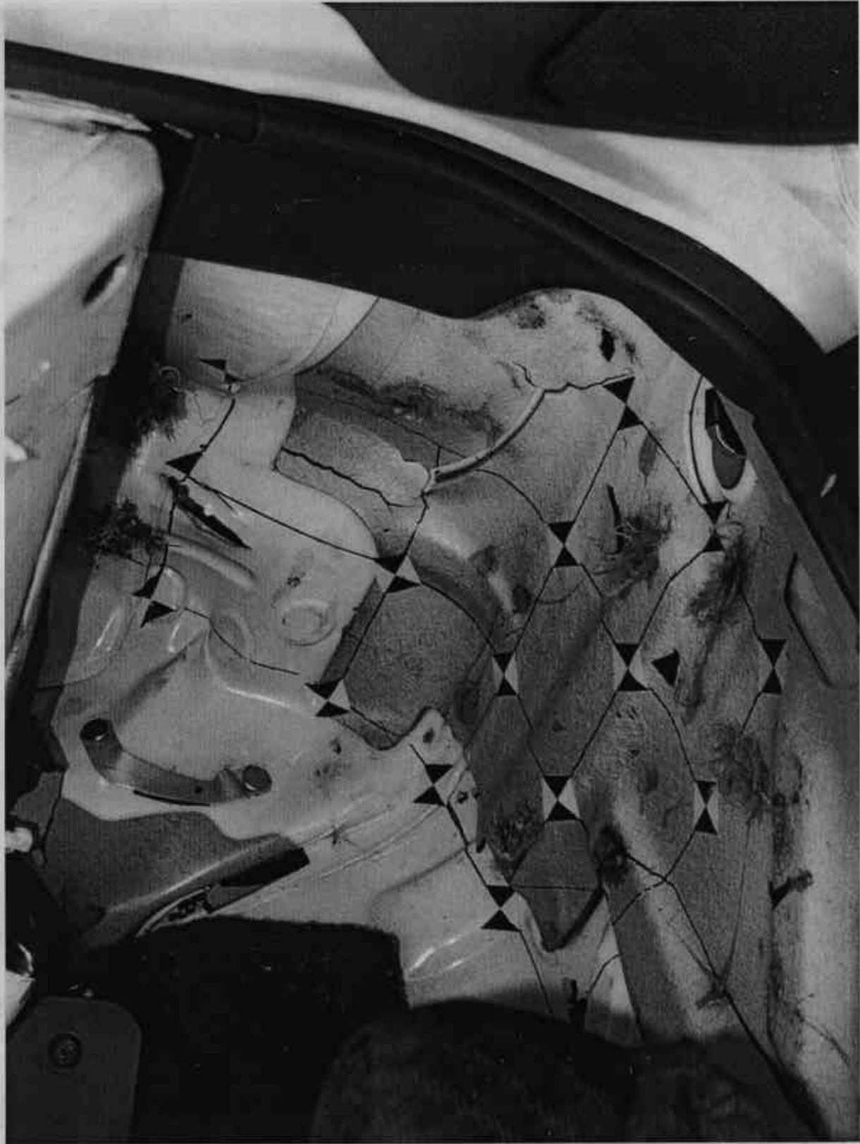
FIGURE A-52. POST TEST PASSENGER SIDE FLOOR PAN
