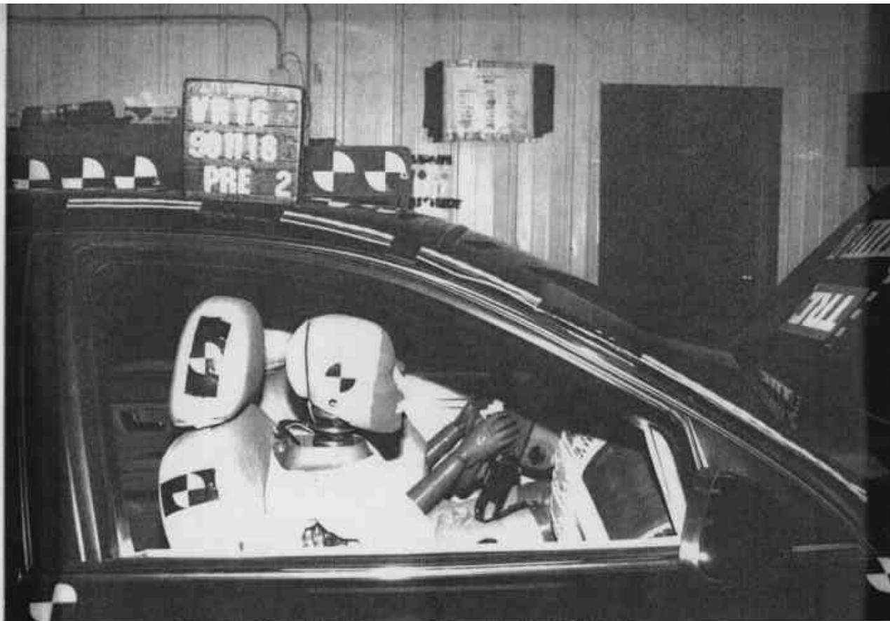
Figure A-35 Pre-Test Passenger Dummy Position - View 1
