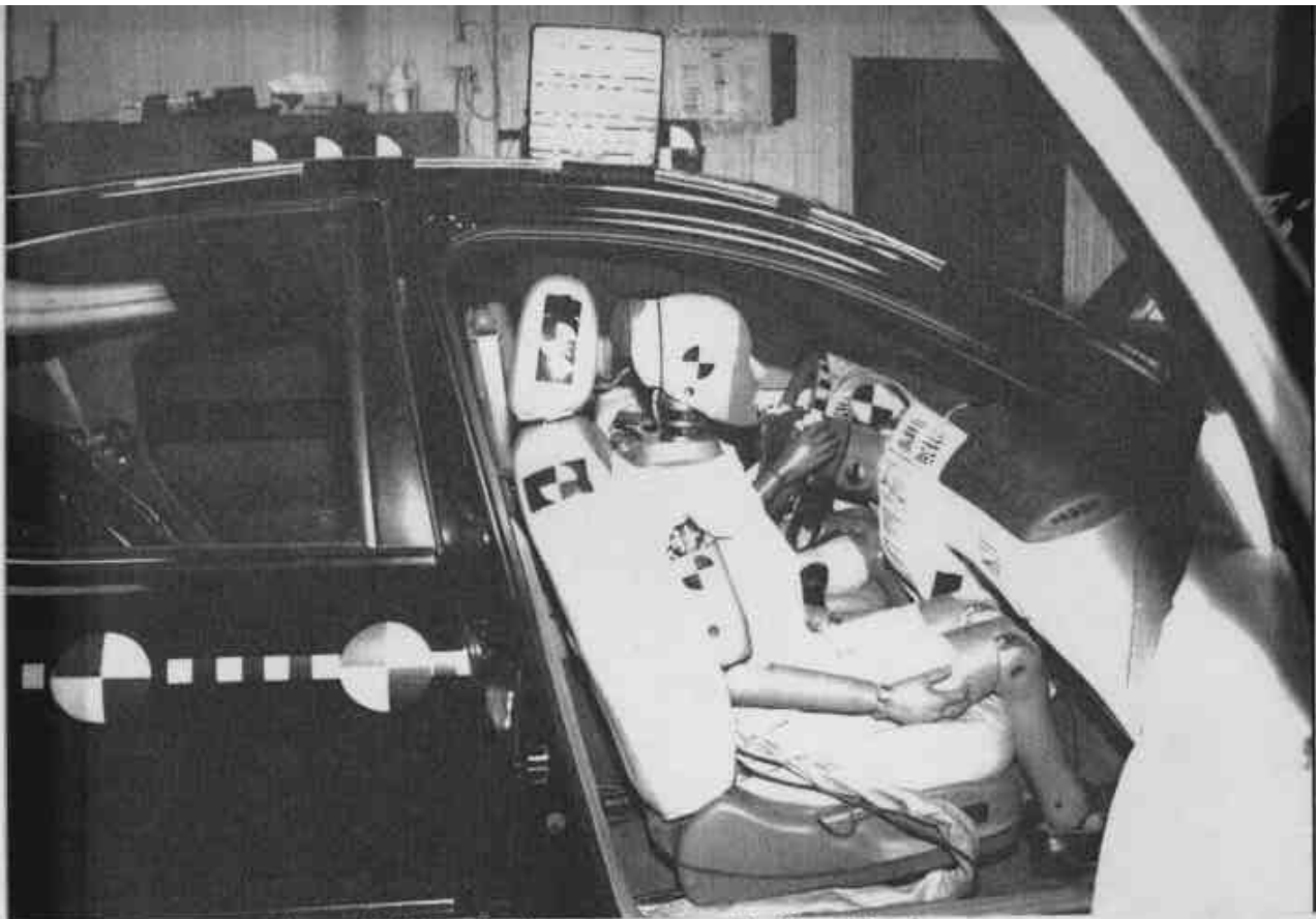
Figure A-37 Pre-Test Passenger Dummy Position - View 2
