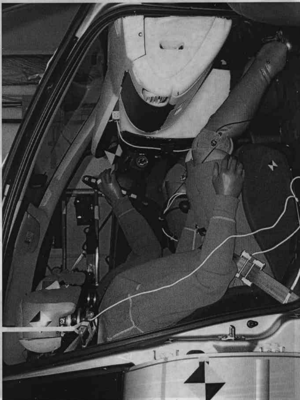
FIGURE A-47. PRE TEST PASSENGER DUMMY (90° TO VEHICLE)
