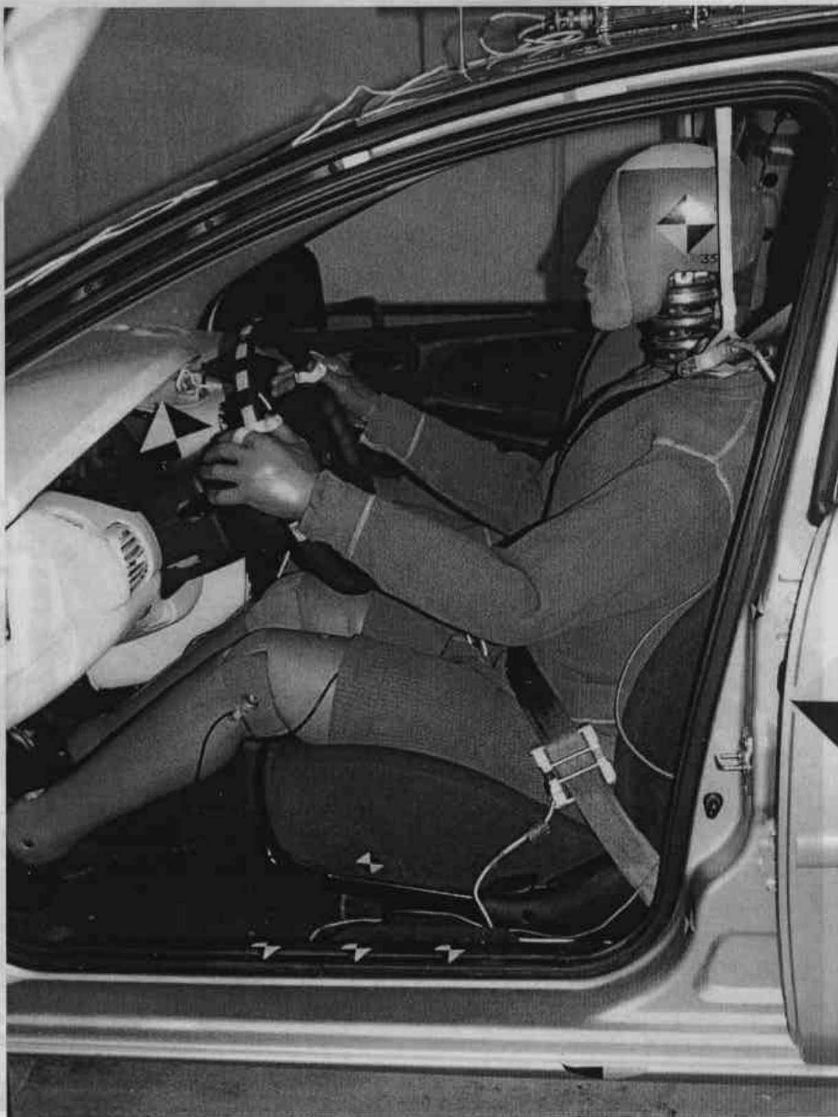
(B) FIGURE A-31. PRETEST DRIVER DUMMY (90° TO VEHICLE)
