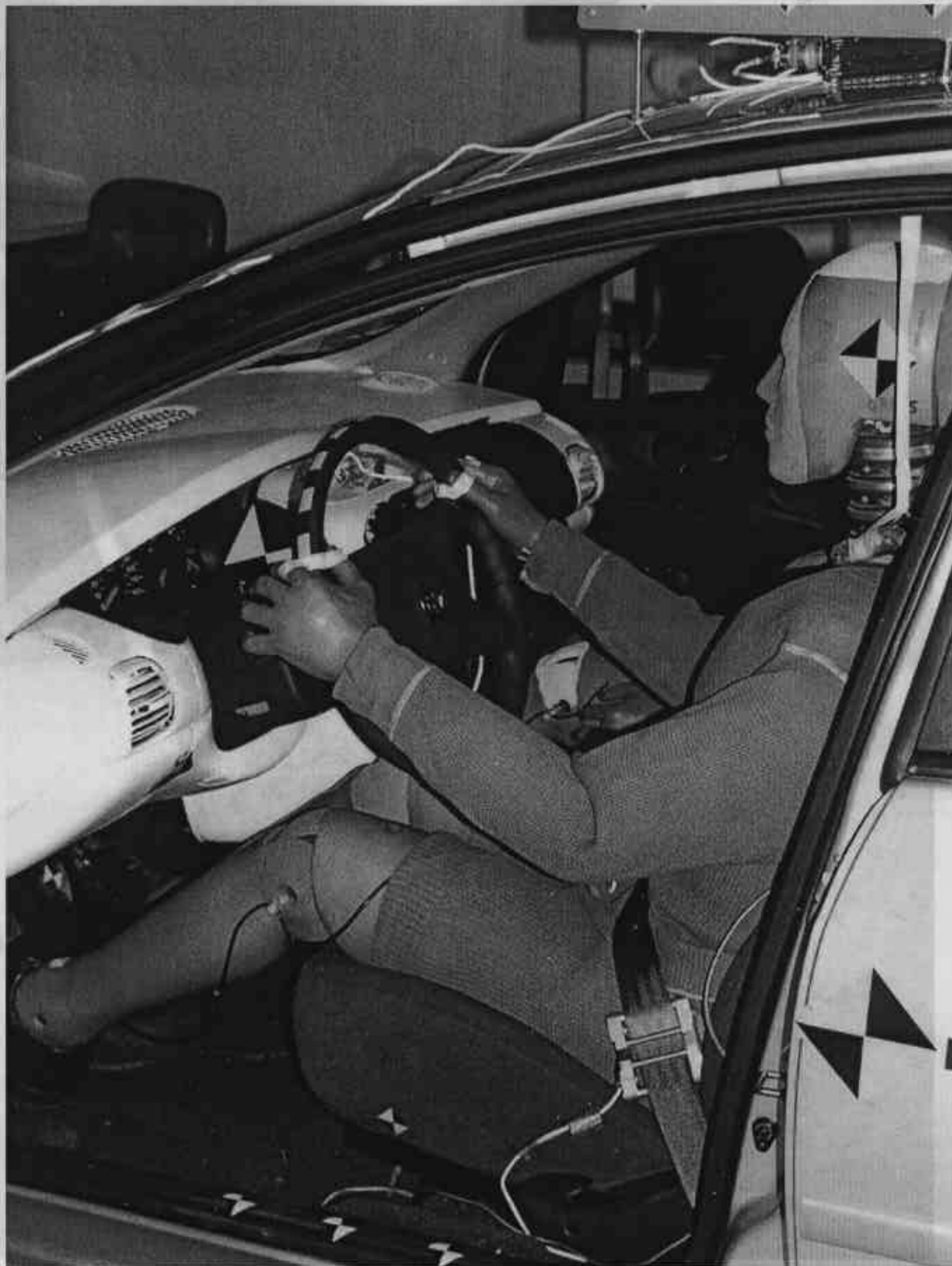
FIGURE A-29. PRETEST DRIVER DUMMY (DOOR OPEN)
