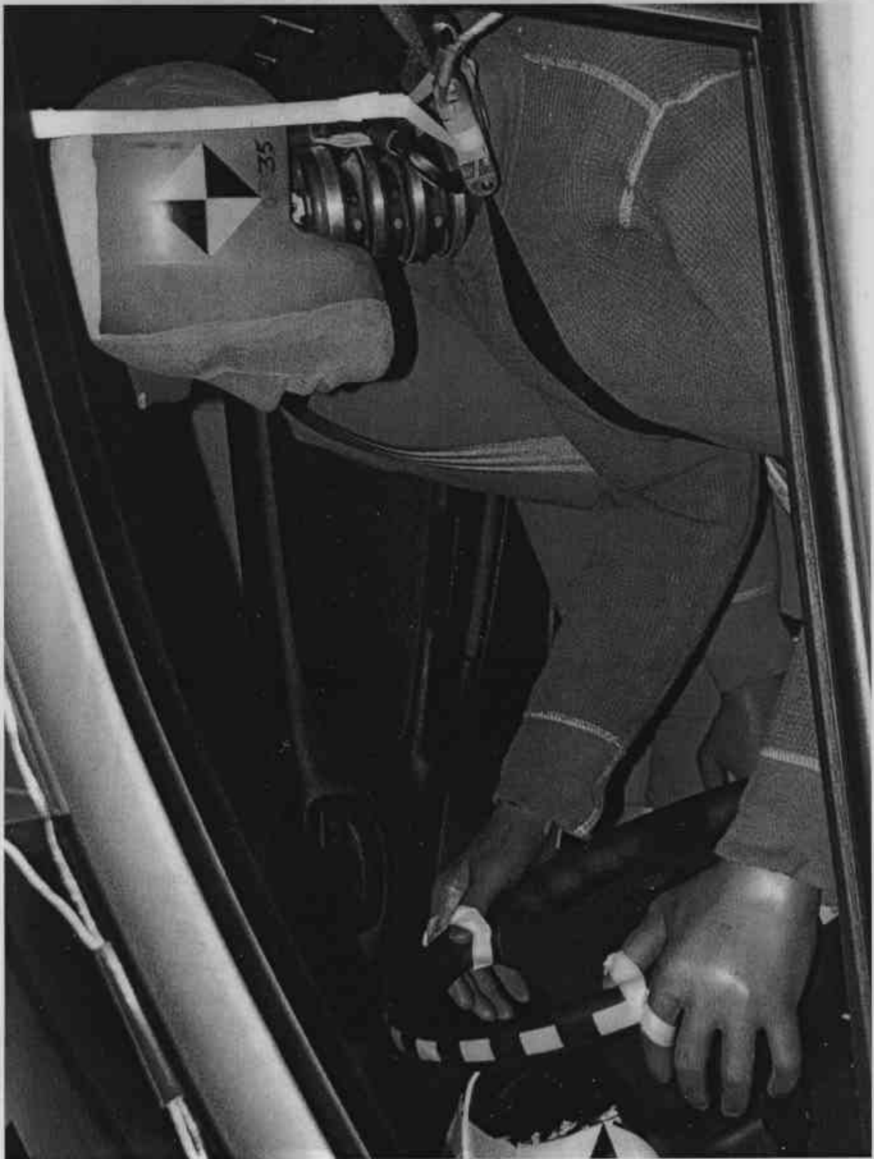
FIGURE A-27. PRETEST DRIVER DUMMY (THRU WINDOW)
