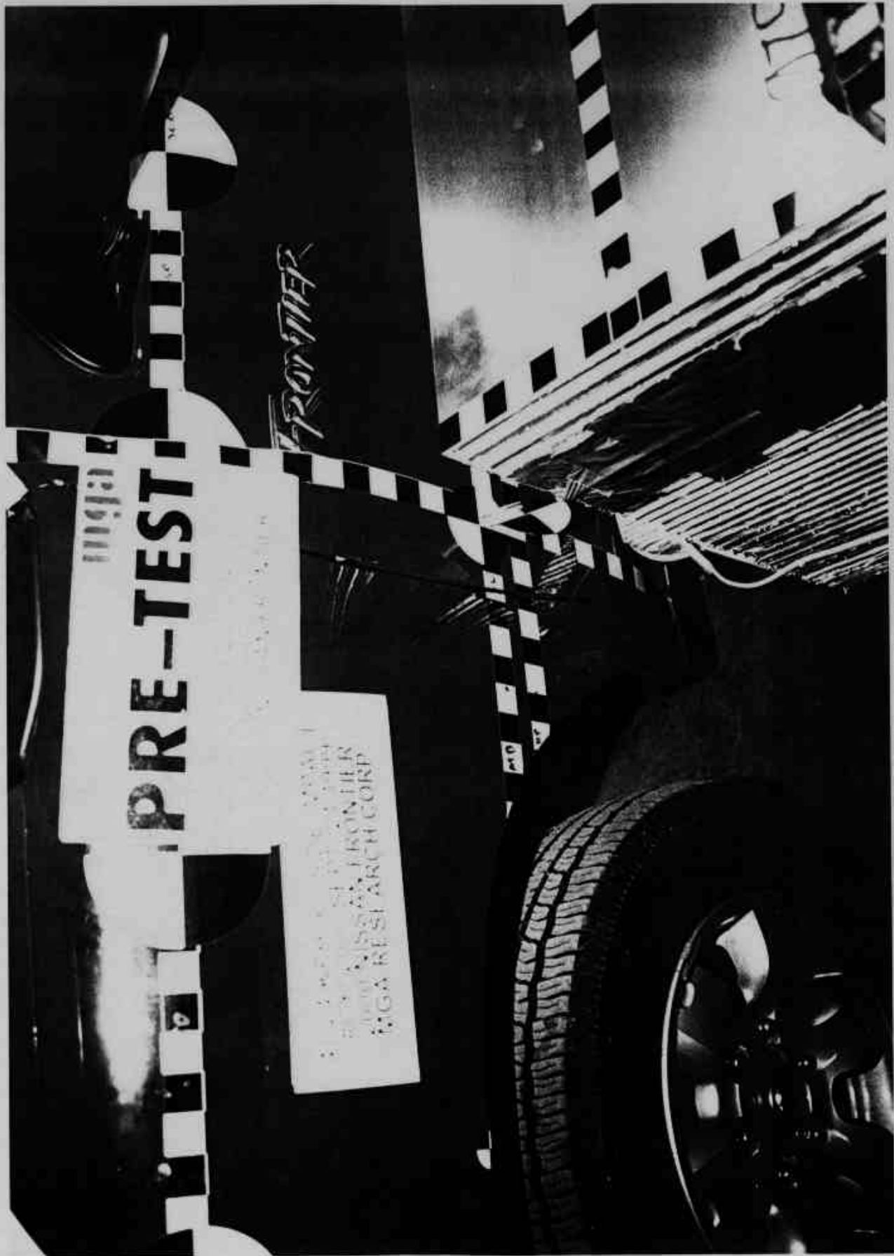
Photo No. A-30 - Pre-Test Right Front Impact Point on Vehicle
