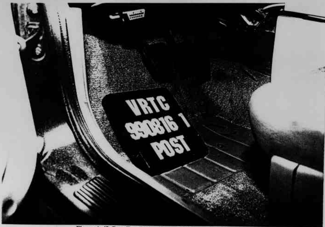
Figure A-49 Post-Test Driver Footwell Deformation View
