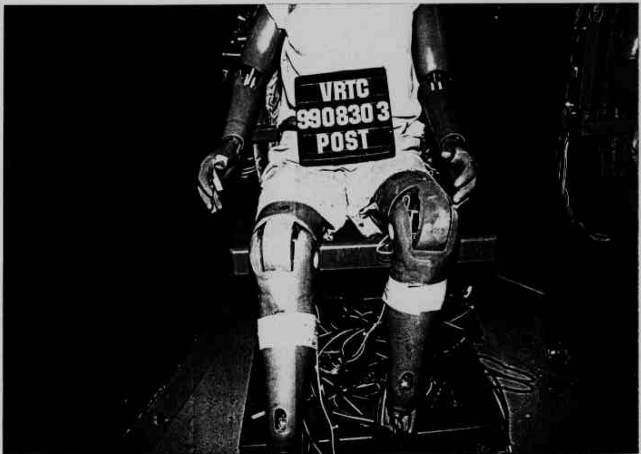
Figure A-48 Post-Test Driver Dummy Knee Contact - View 1
