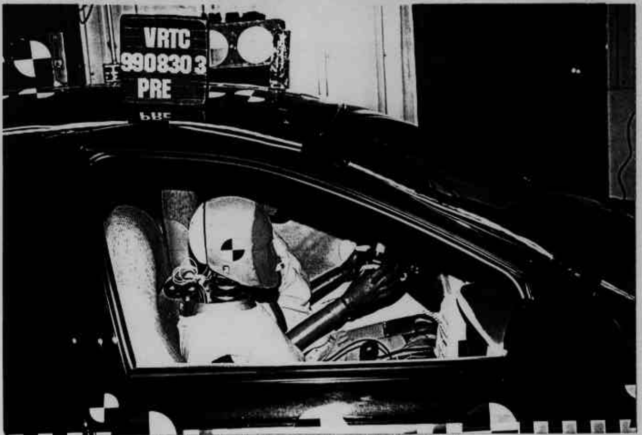
Figure A-37 Pre-Test Passenger Dummy Position - View 1
