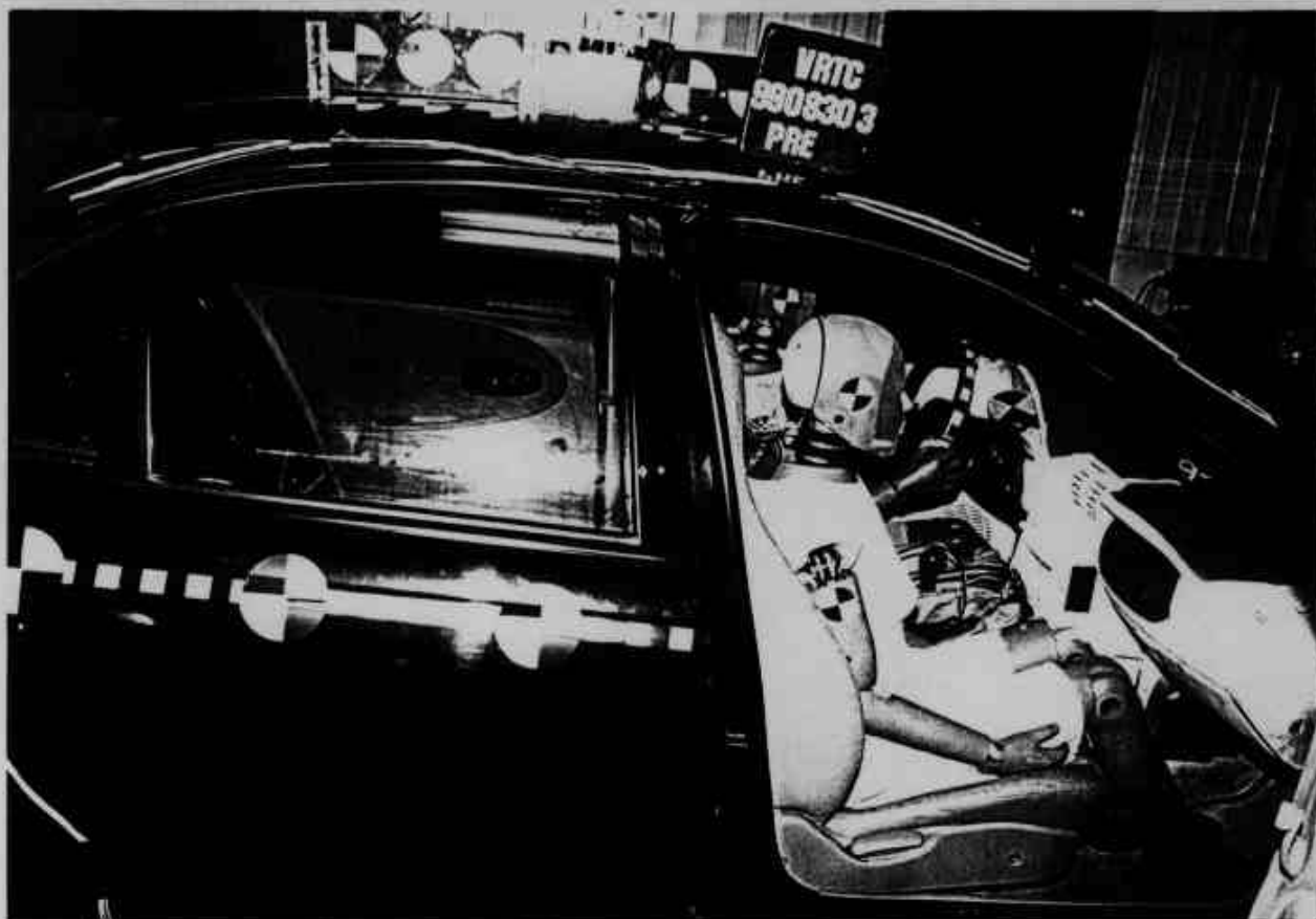
Figure A-39 Pre-Test Passenger Dummy Position - View 2
