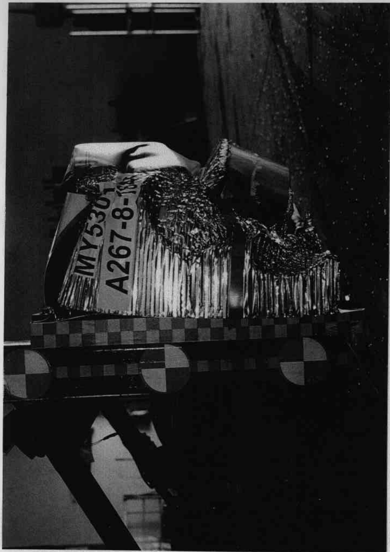
Figure A-12 POST-TEST RIGHT SIDE VIEW OF IMPACTOR FACE
