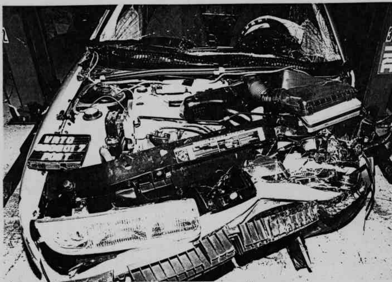
Figure A-26 Post-Test Engine Compartment View
