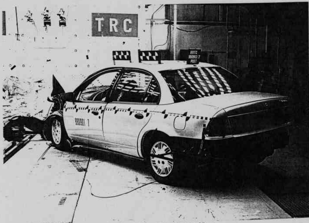
Figure A-6 Post-Test Left Rear Three-Quarter View
