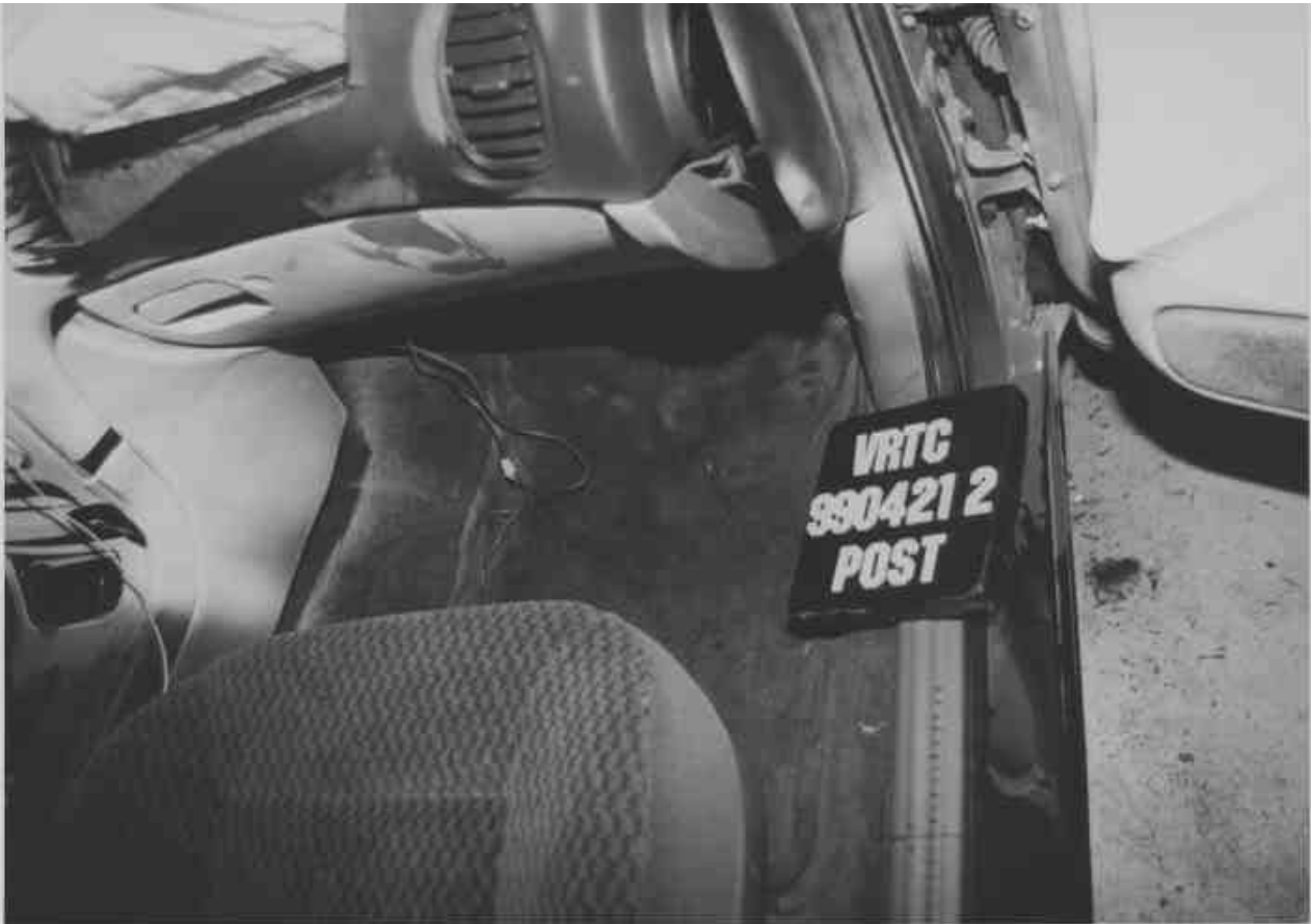
Figure A-54 Post-Test Passenger Footwell Deformation View
