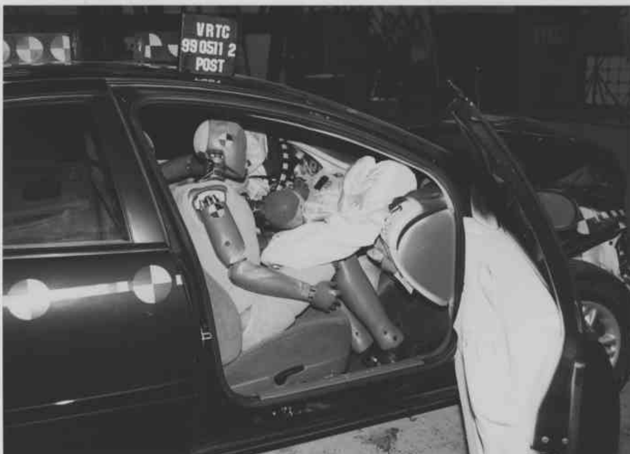
Figure A-44 Post-Test Passenger Dummy Position - View 2
