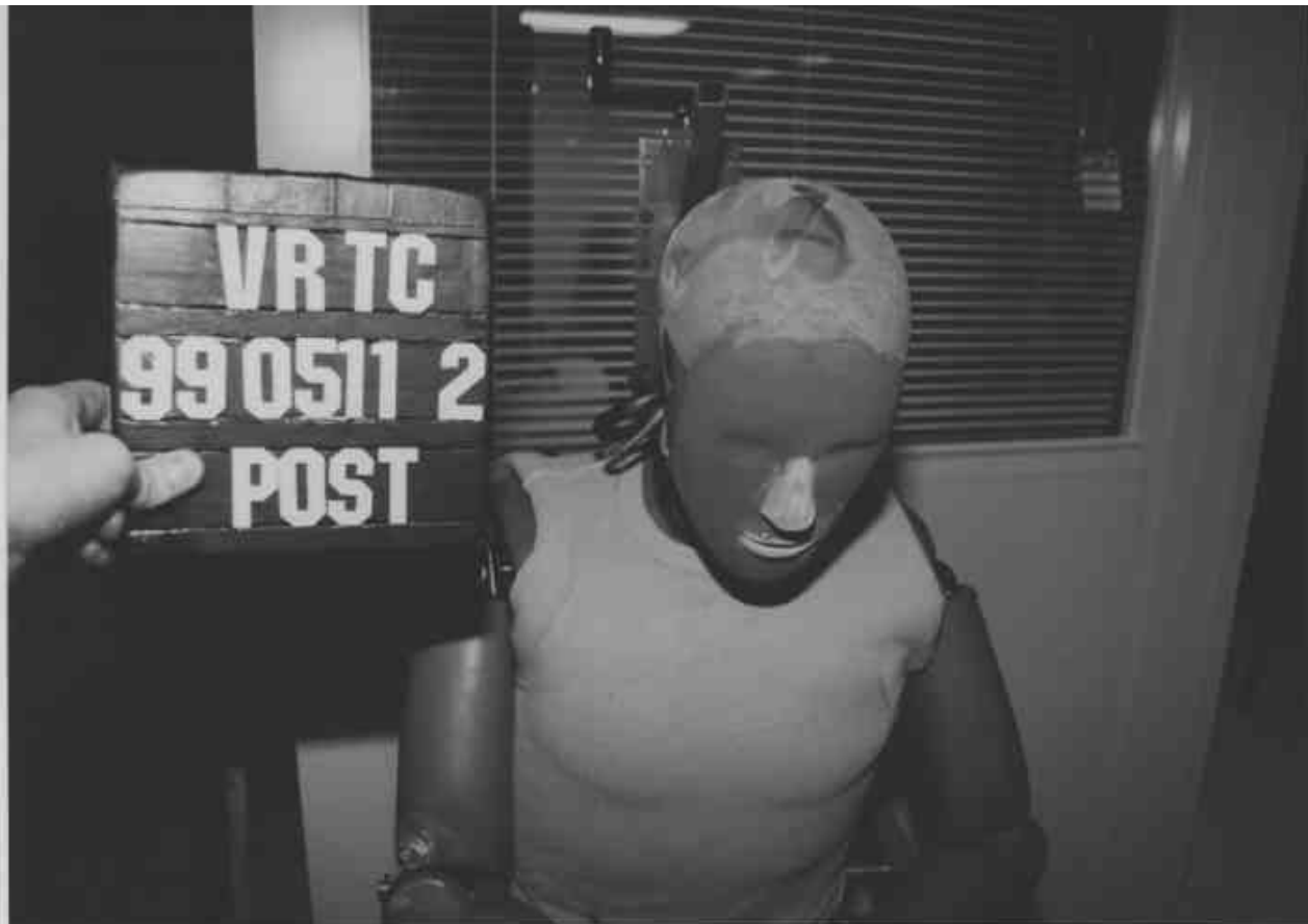
Figure A-53 Post-Test Passenger Dummy Head Contact - View 1
