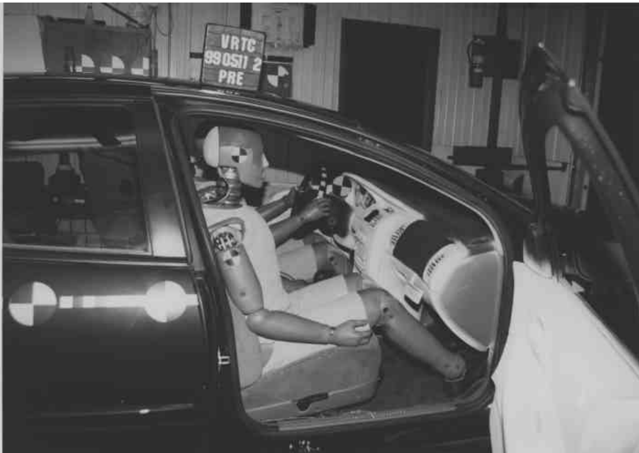
Figure A-43 Pre-Test Passenger Dummy Position - View 2
