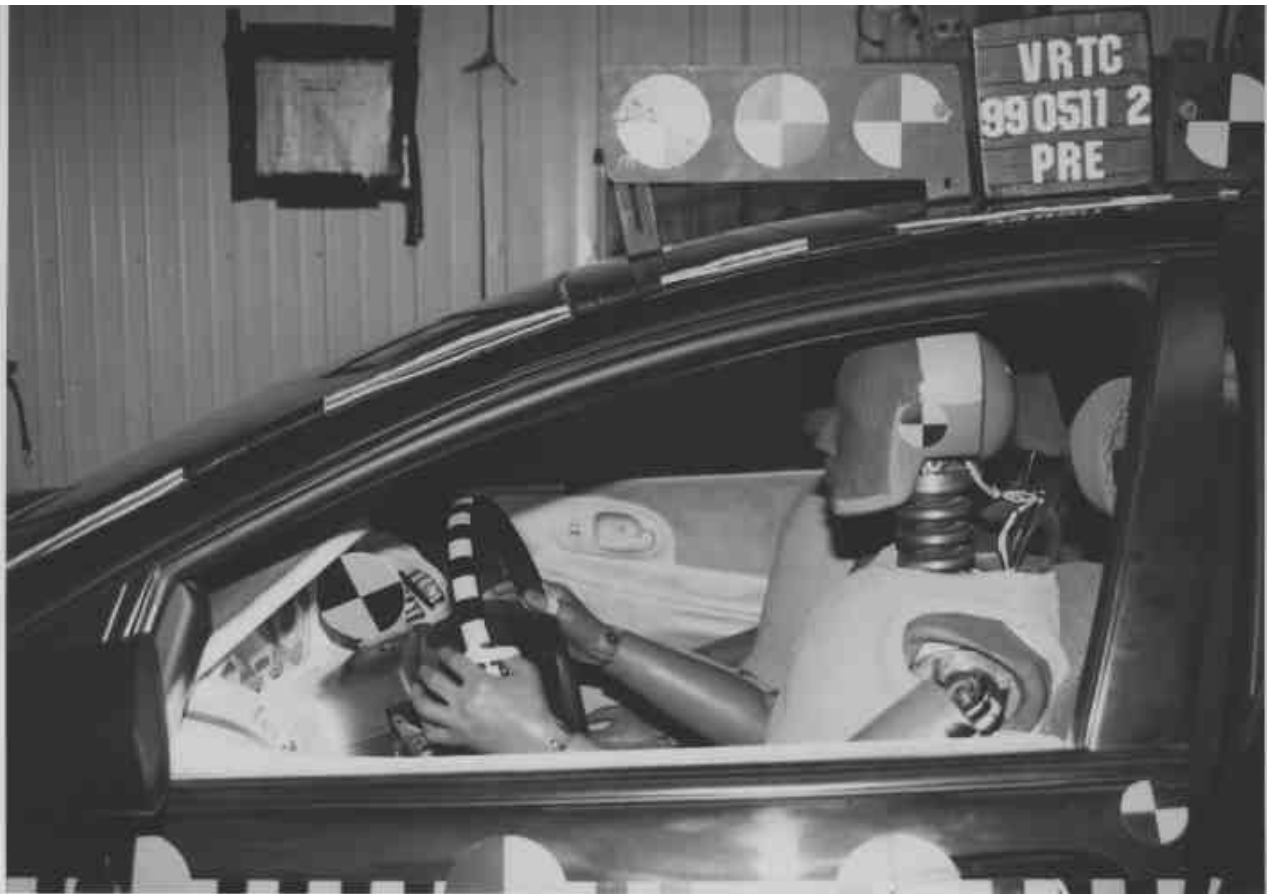
Figure A-35 Pre-Test Driver Dummy Position - View 1
