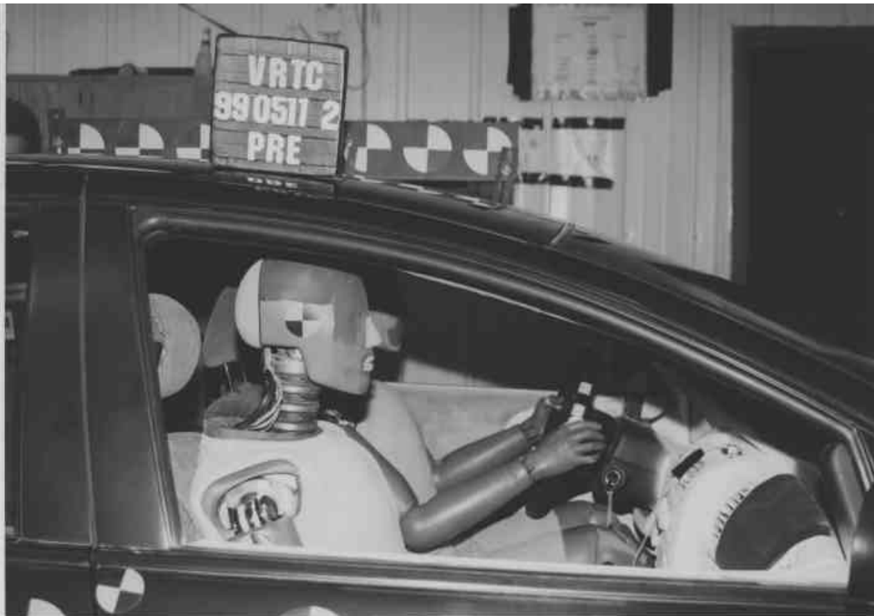
Figure A-41 Pre-Test Passenger Dummy Position - View 1
