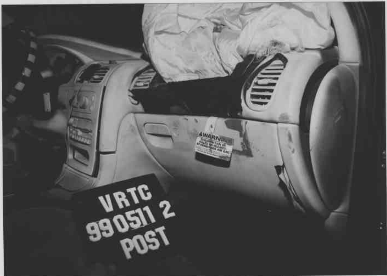
Figure A-56 Post-Test Passenger Dummy Knee Contact - View 2
