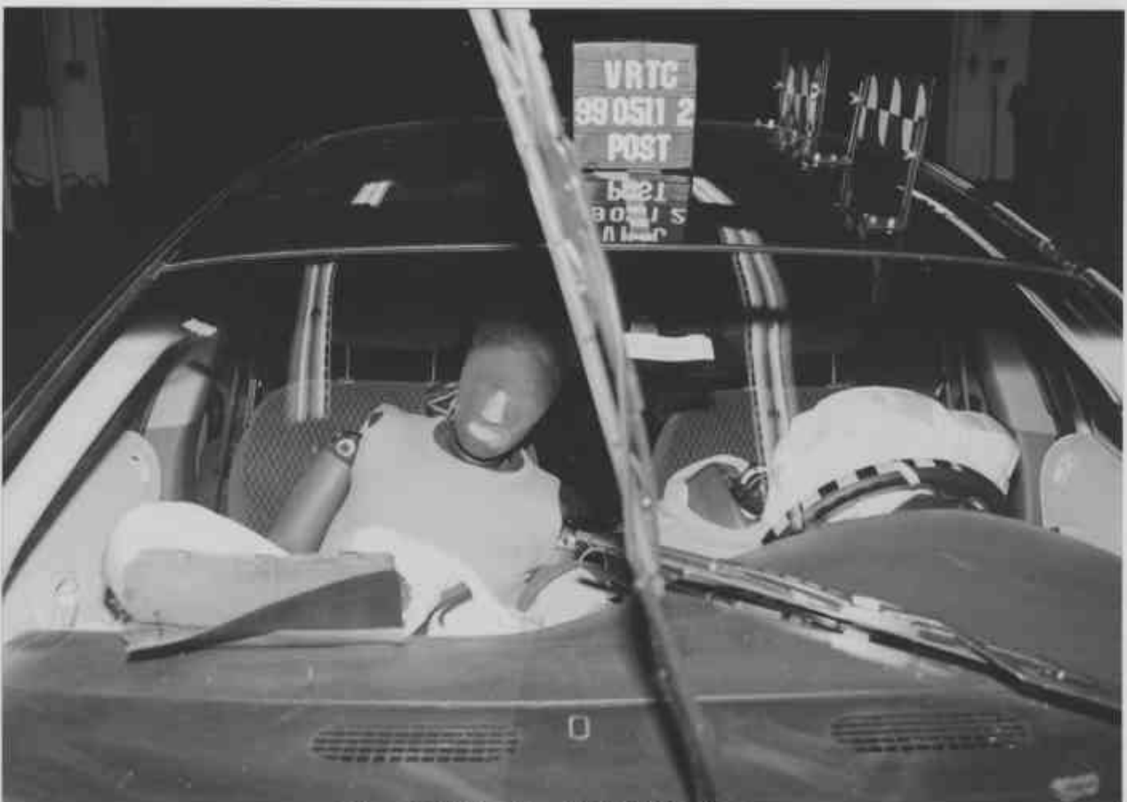
Figure A-30 Post-Test Windshield - View 2
