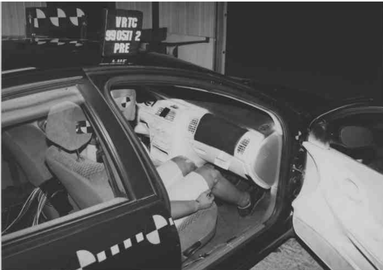
Figure A-45 Pre-Test Passenger Dummy Position - View 3
