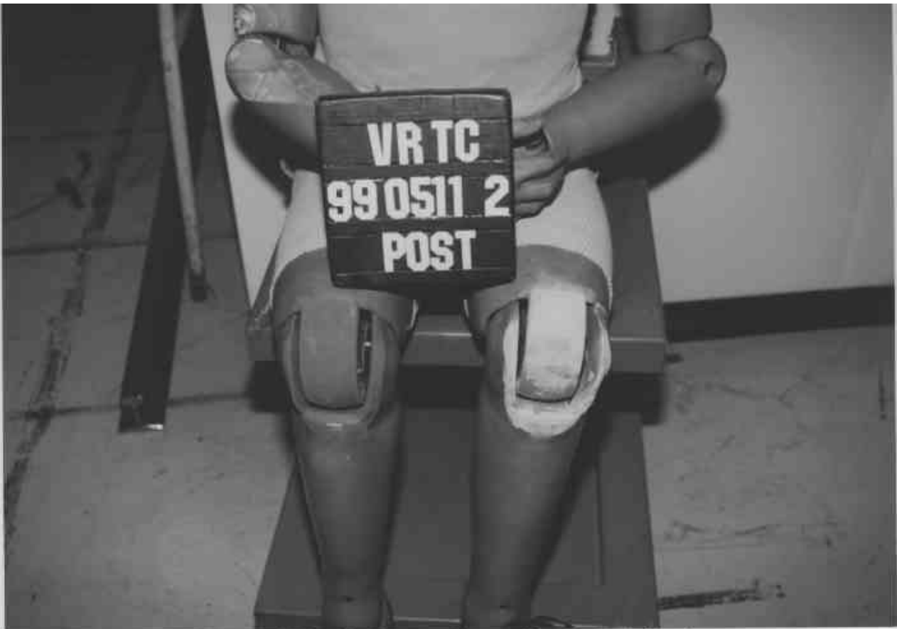
Figure A-55 Post-Test Passenger Dummy Knee Contact - View 1
