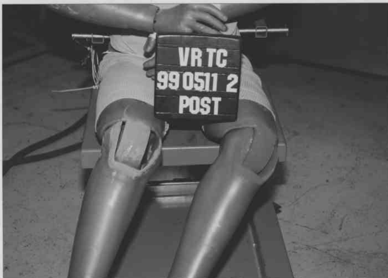
Figure A-50 Post-Test Driver Dummy Knee Contact - View 1
