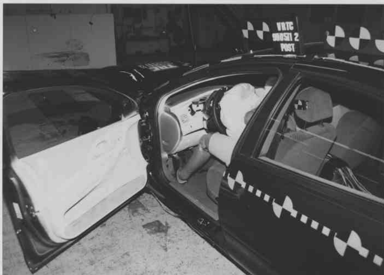
Figure A-40 Post-Test Driver Dummy Position - View 3
