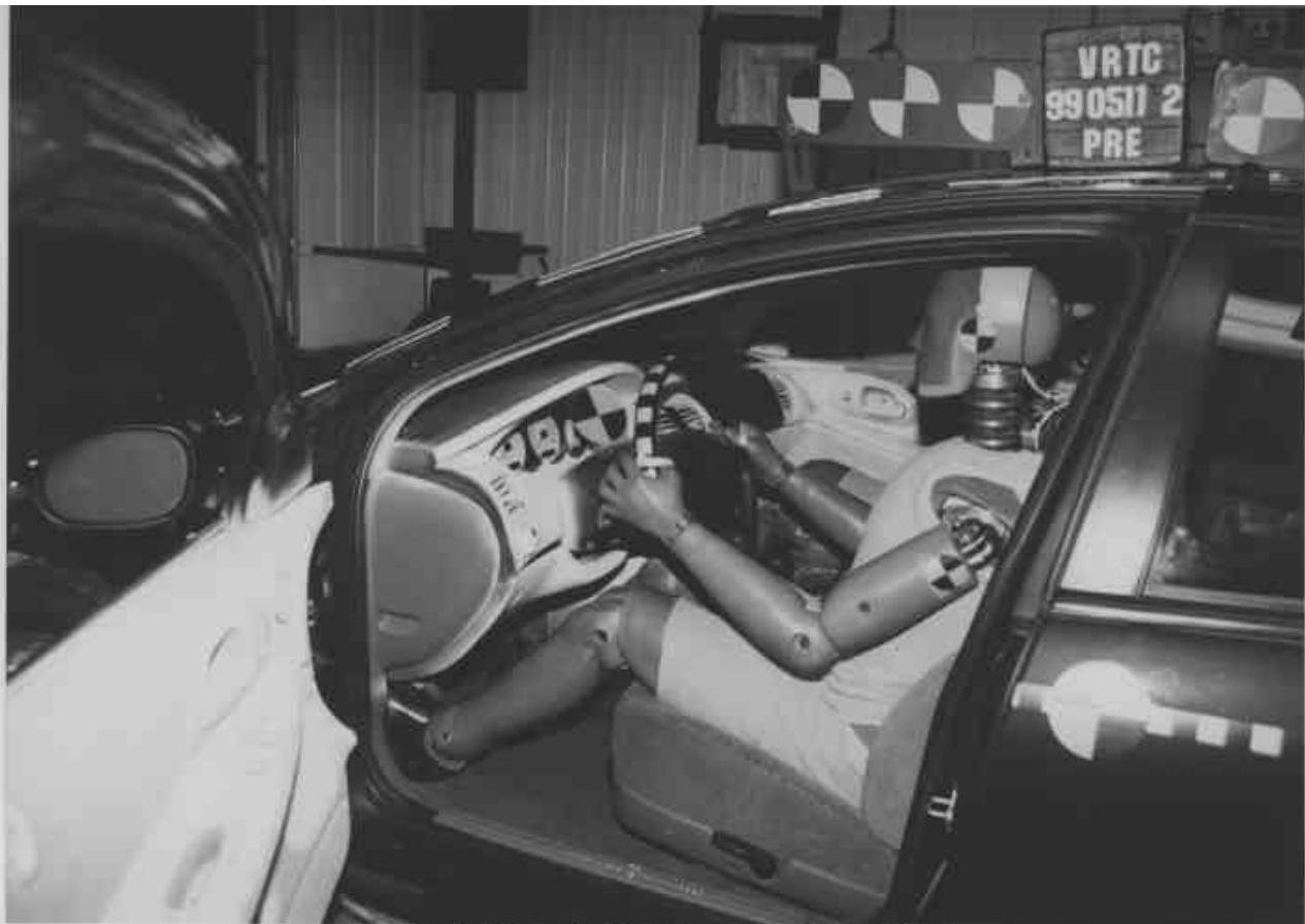
Figure A-37 Pre-Test Driver Dummy Position -View 2
