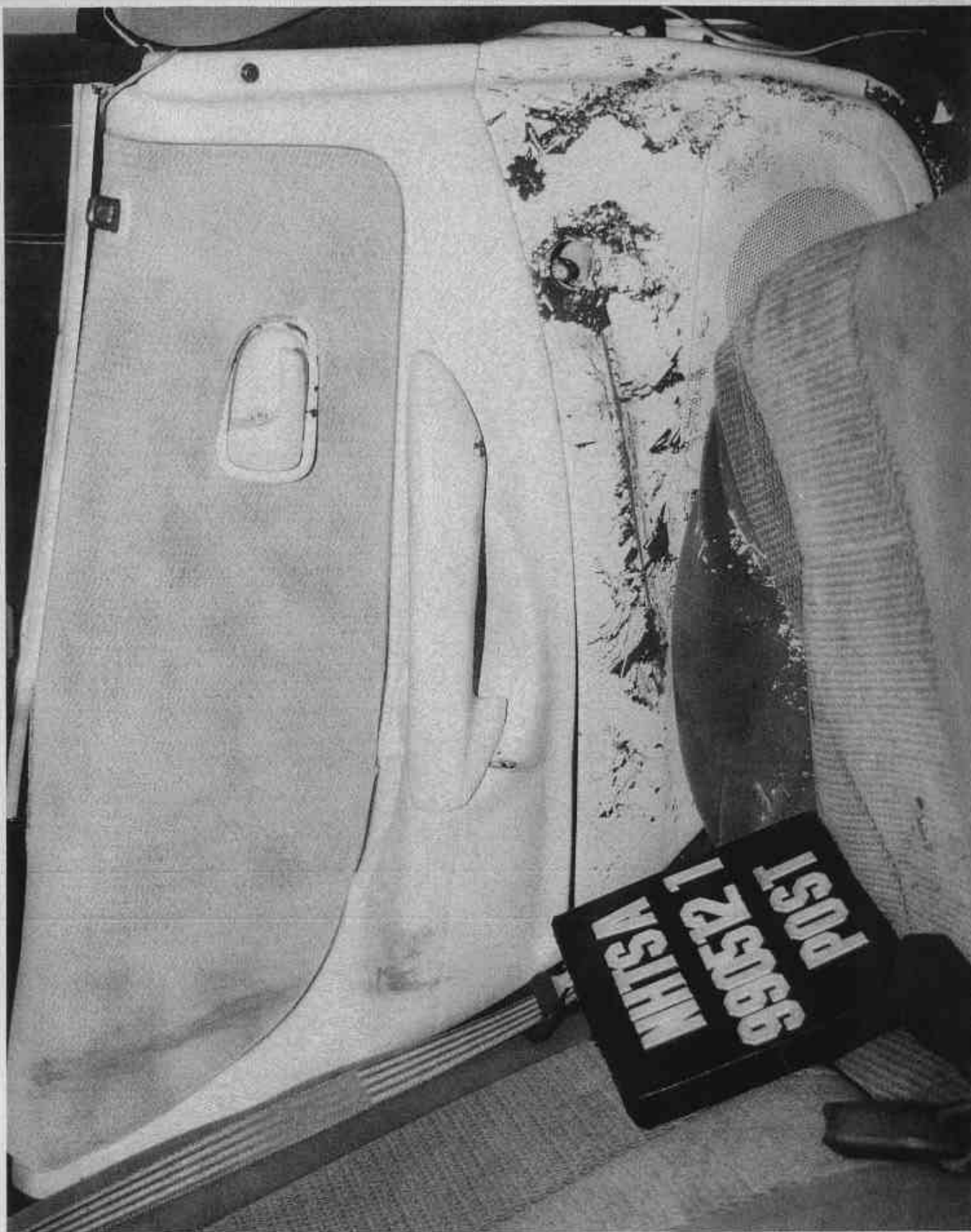
Figure A-28 Post-Test Interior of Rear Panel Showing SID Impact Locations A-30 990512
