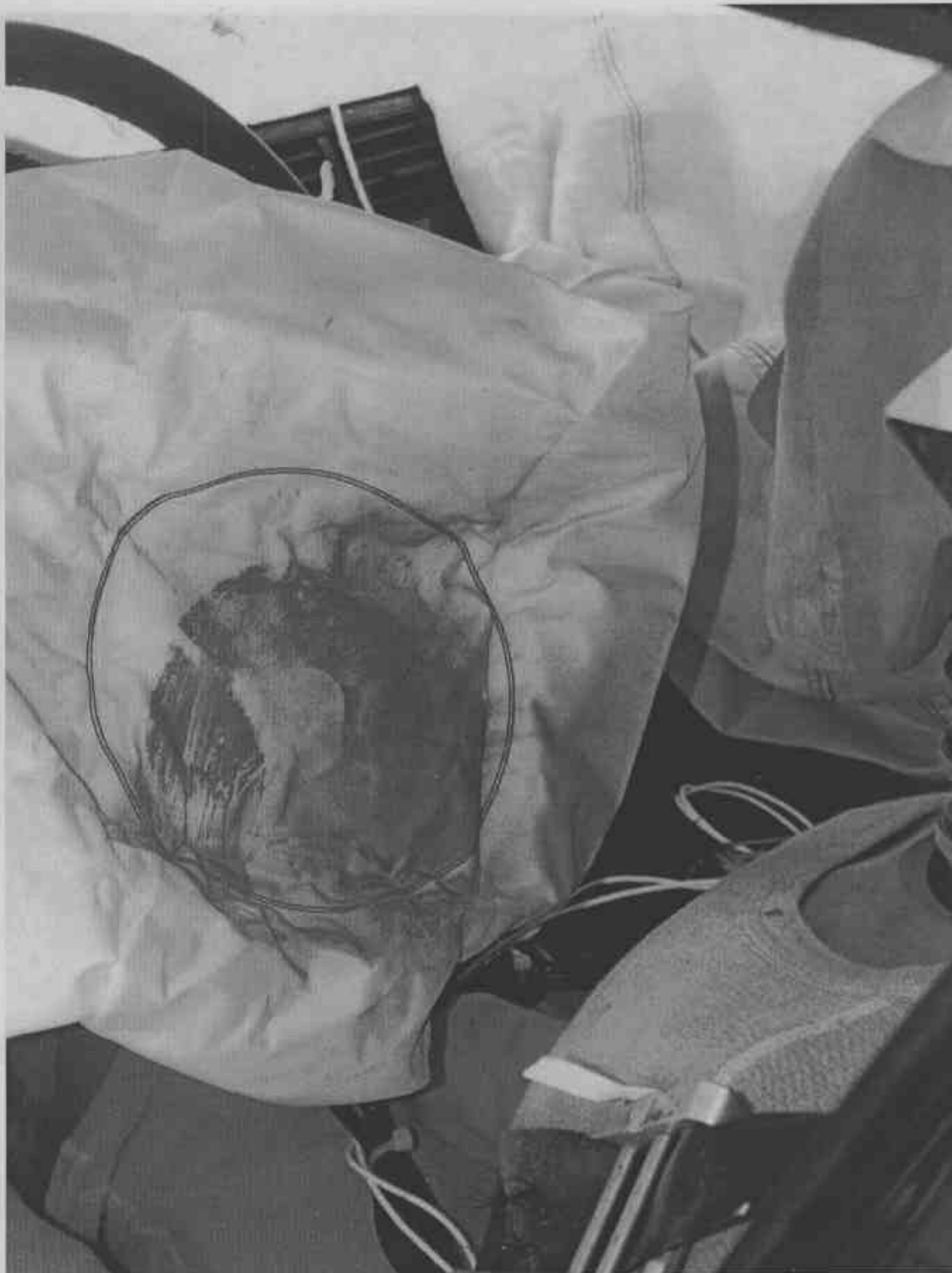
FIGURE A-40. POST TEST DRIVER DUMMY CONTACT
