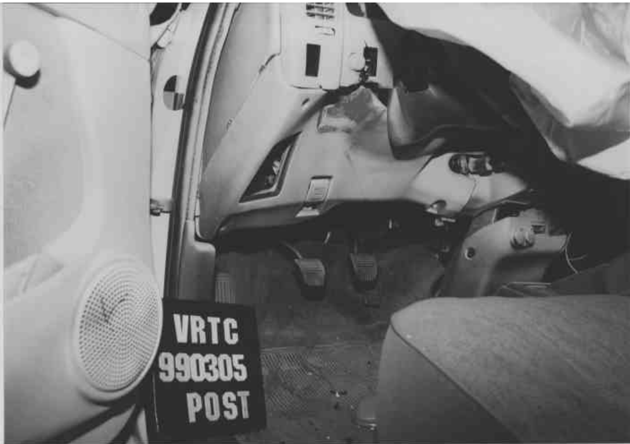
Figure A-45 Post-Test Driver Footwell Deformation View
