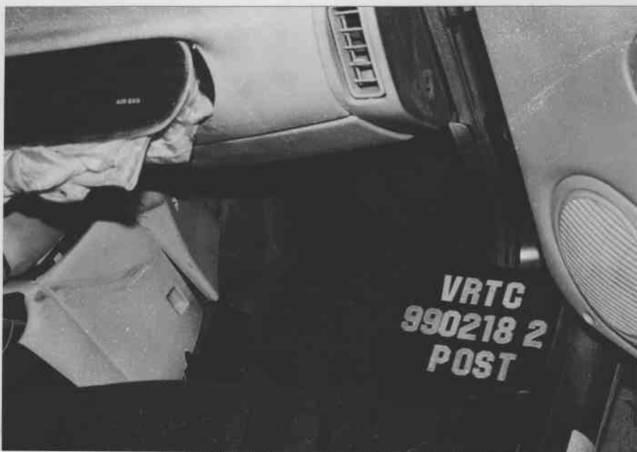
Figure A-48 Post-Test Passenger Footwell Deformation View
