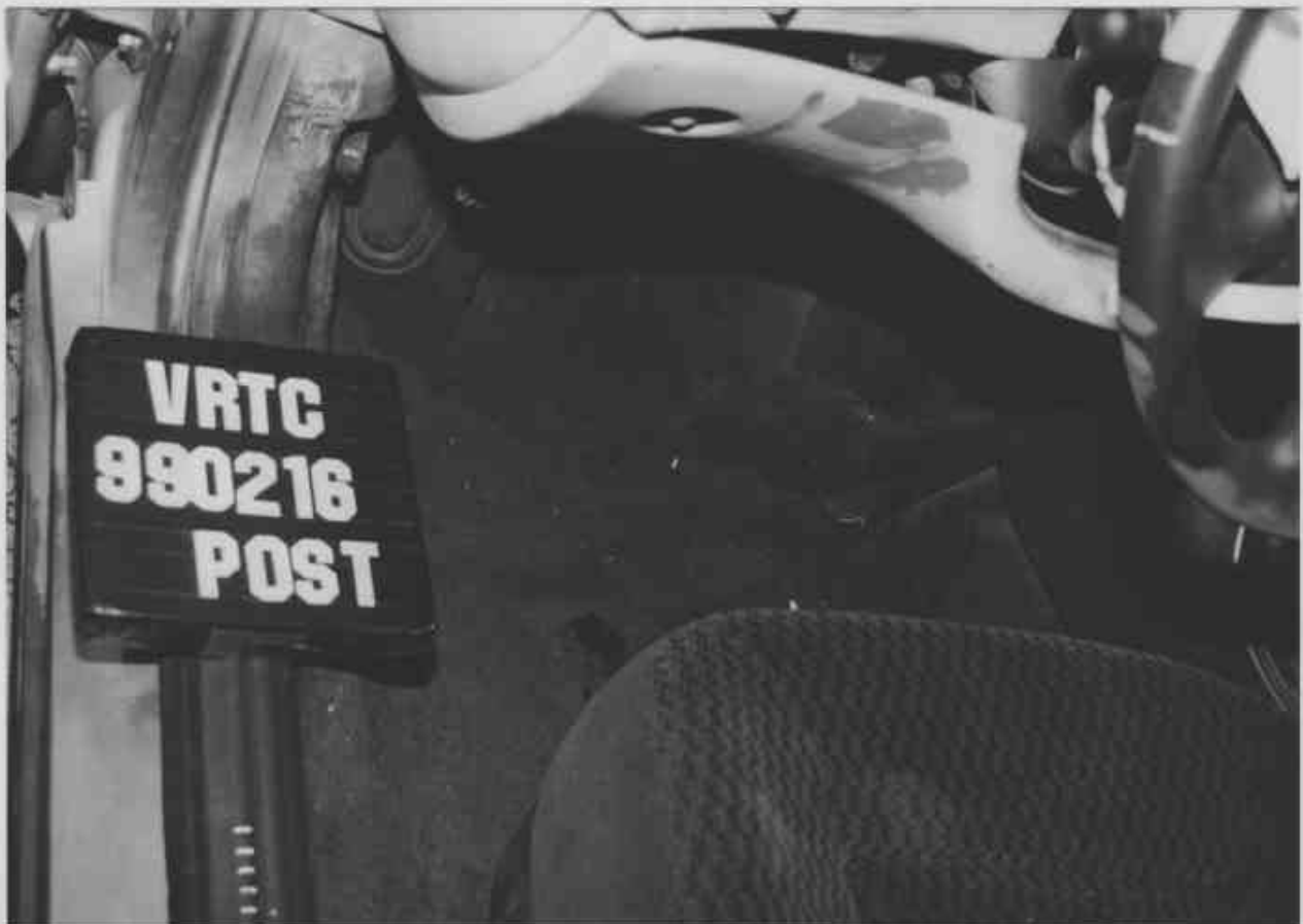
Figure A-42 Post-Test Driver Footwell Deformation View
