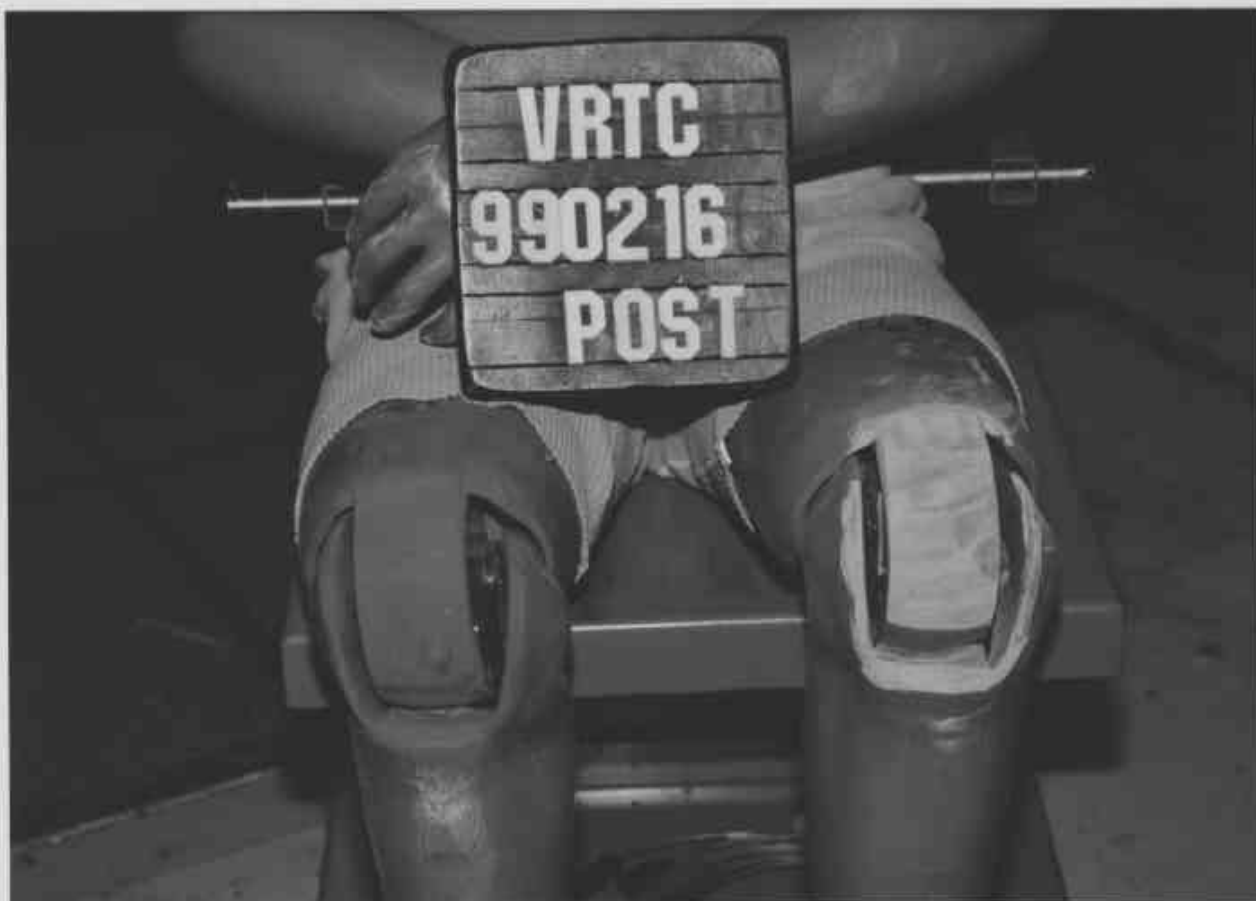
Figure A-46 Post-Test Passenger Dummy Knee Contact - View 1
