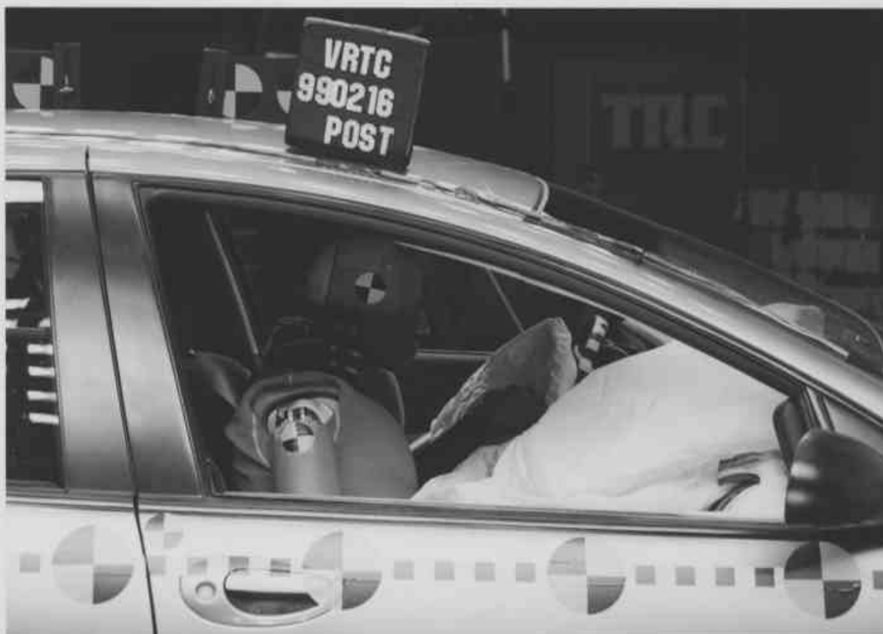
Figure A-32 Post-Test Passenger Dummy Position - View 1
