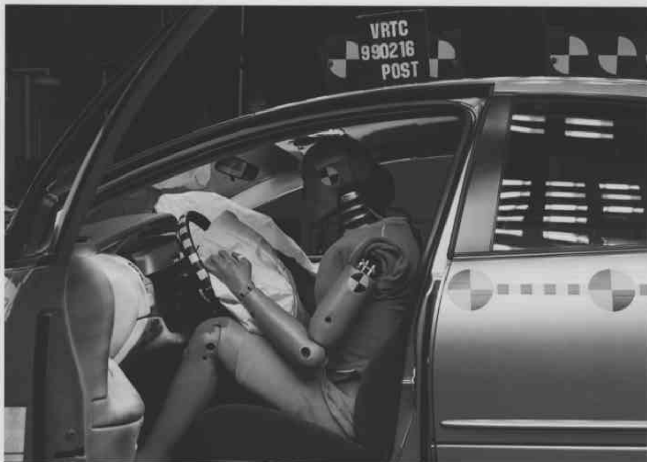
Figure A-28 Post-Test Driver Dummy Position - View 2
