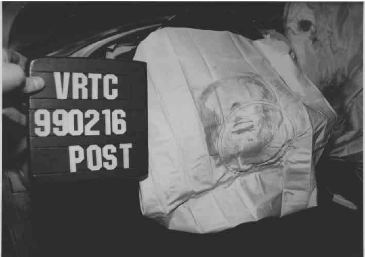
Figure A-39 Post-Test Driver Dummy Head Contact - View 2
