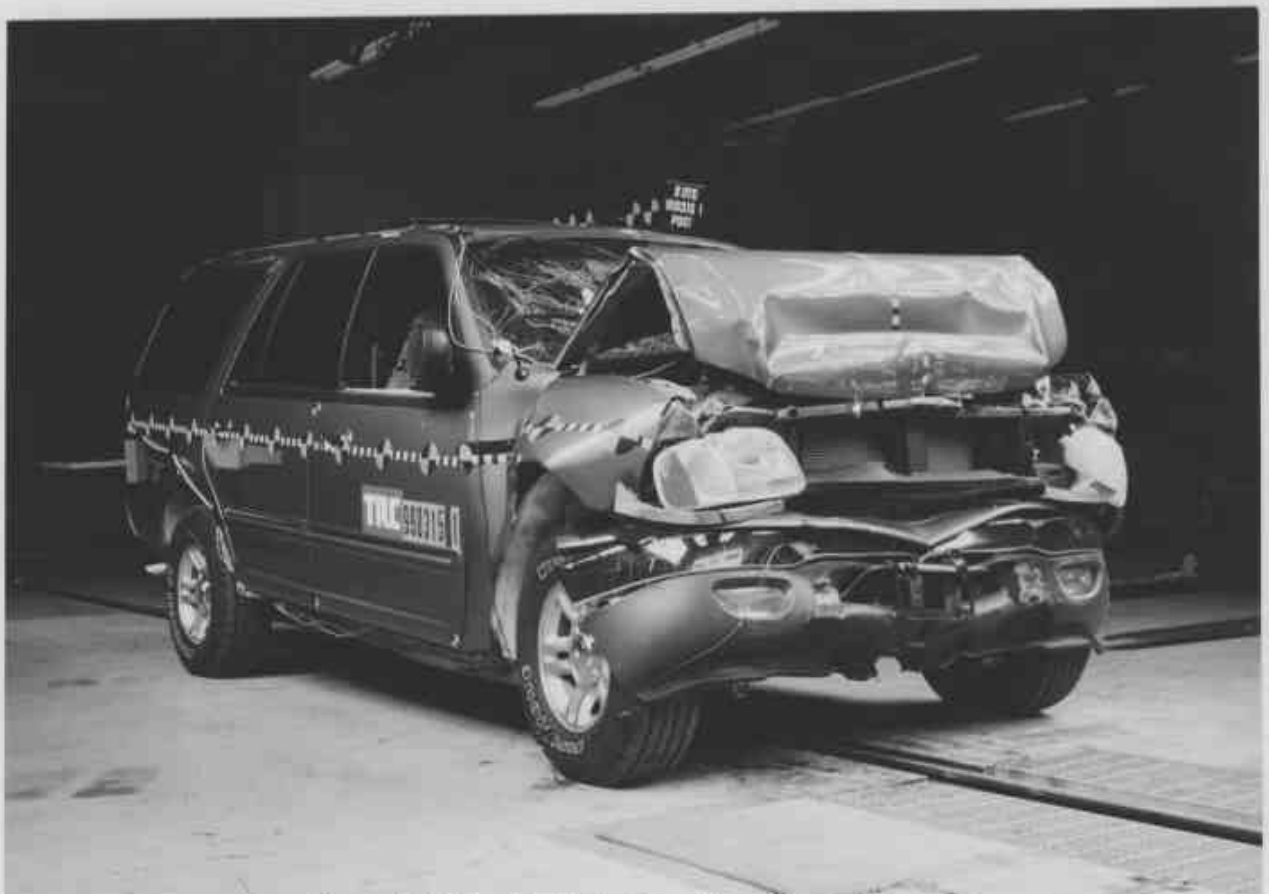
Figure A-12 Post-Test Right Front Three-Quarter View
