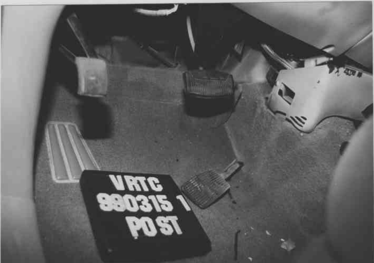
Figure A-43 Post-Test Driver Footwell Deformation View
