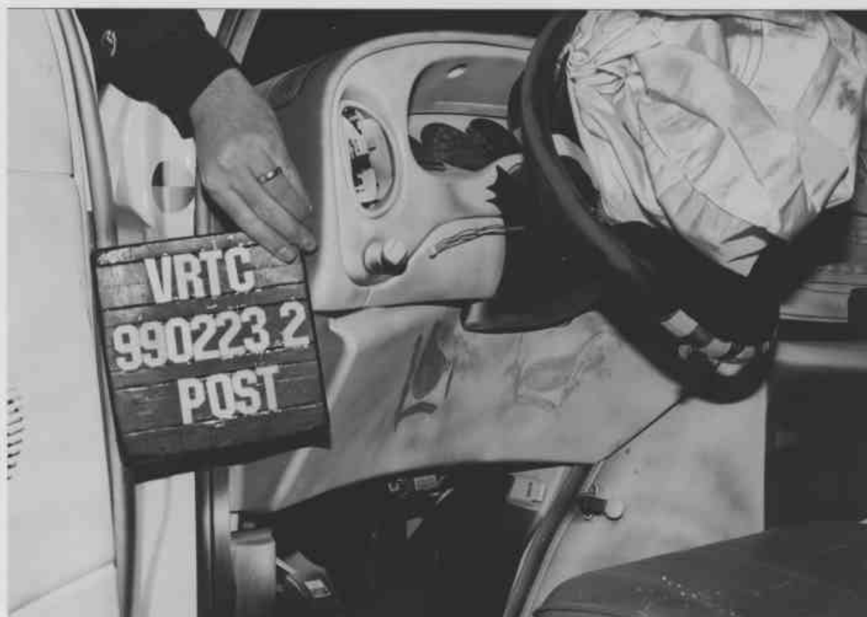
Figure A-50 Post-Test Driver Dummy Knee Contact - View 2
