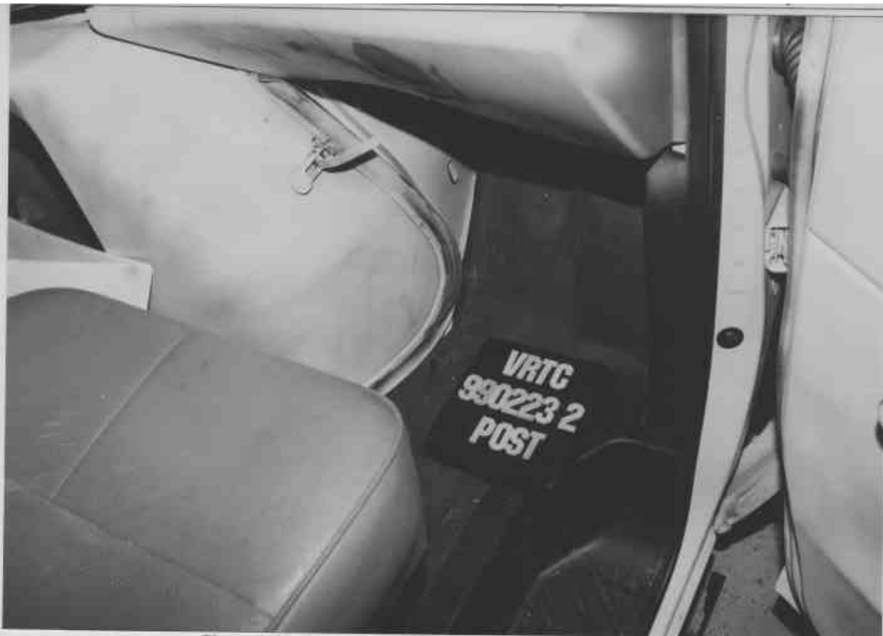
Figure A-57 Post-Test Passenger Footwell Deformation View
