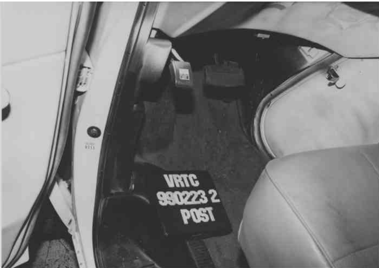
Figure A-51 Post-Test Driver Footwell Deformation View
