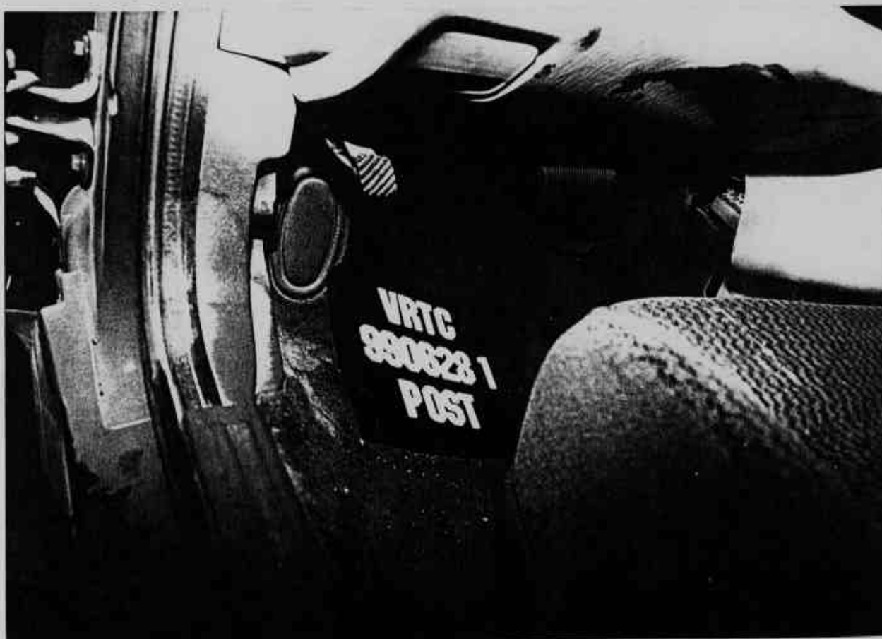
Figure A-56 Post-Test Driver Footwell Deformation View
