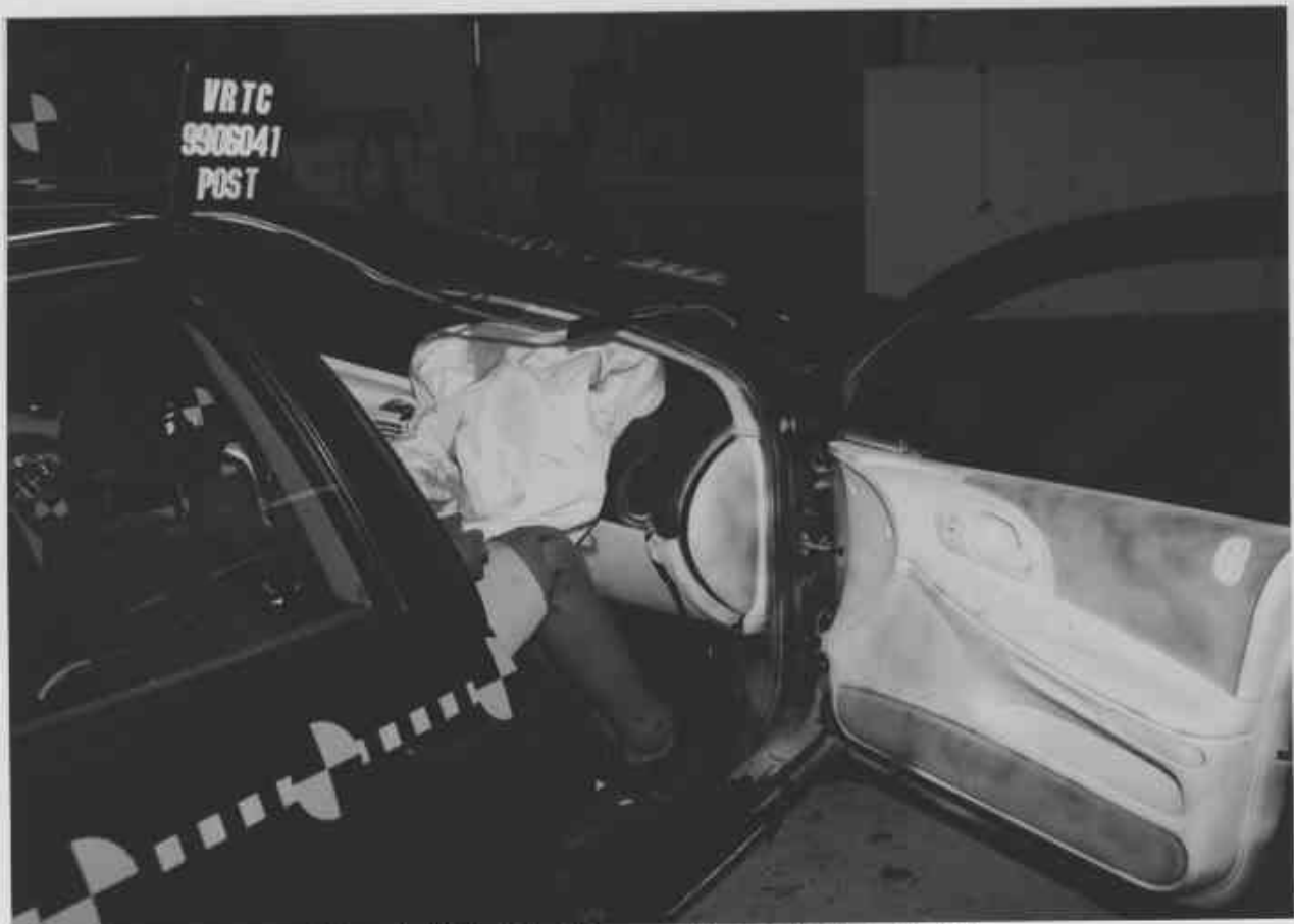
Figure A-50 Post-Test Passenger Dummy Position - View 3
