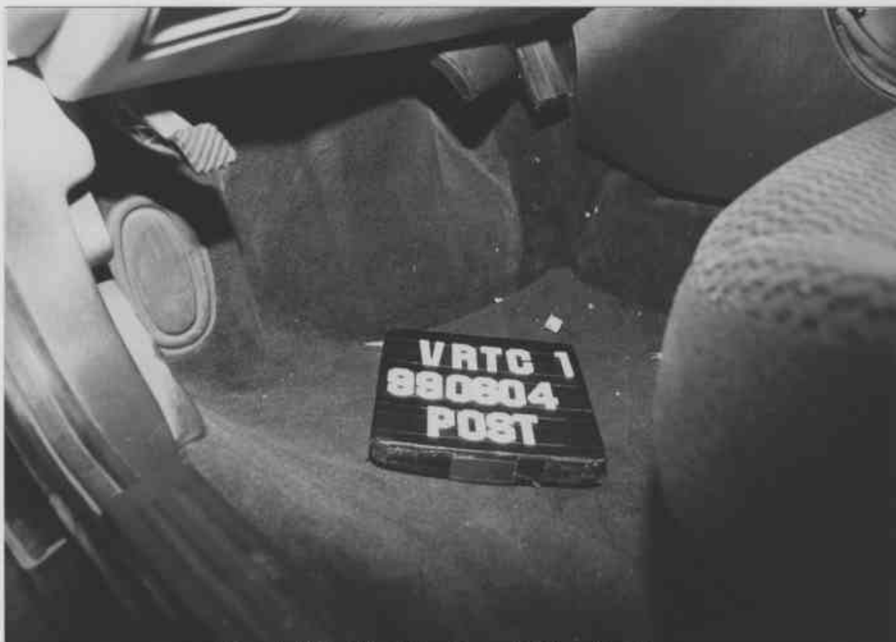
Figure A-58 Post-Test Driver Footwell Deformation View
