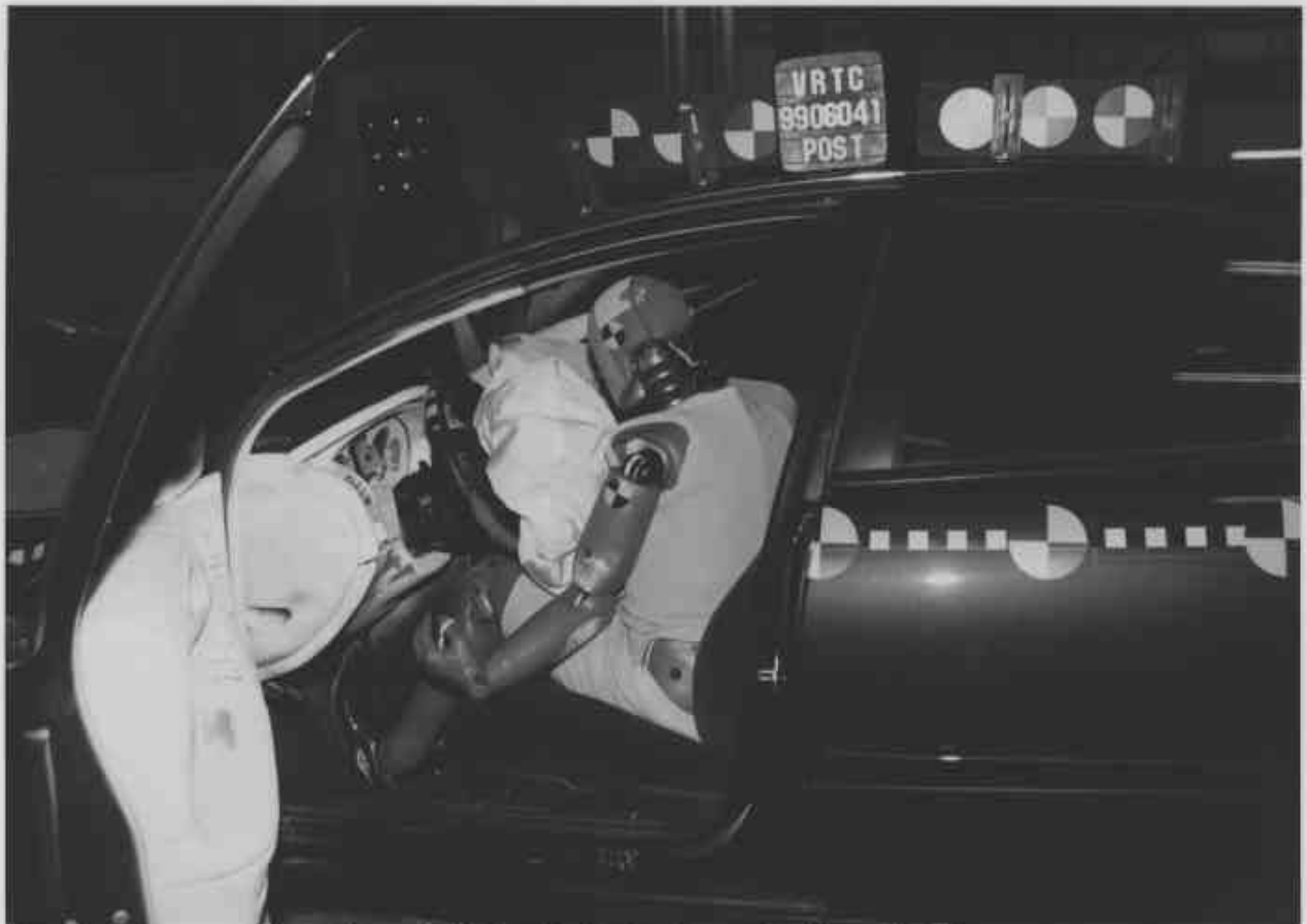
Figure A-42 Post-Test Driver Dummy Position - View 2
