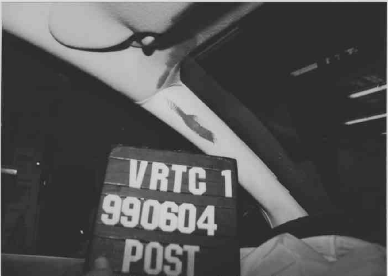
Figure A-54 Post-Test Driver Dummy Head Contact - View 3
