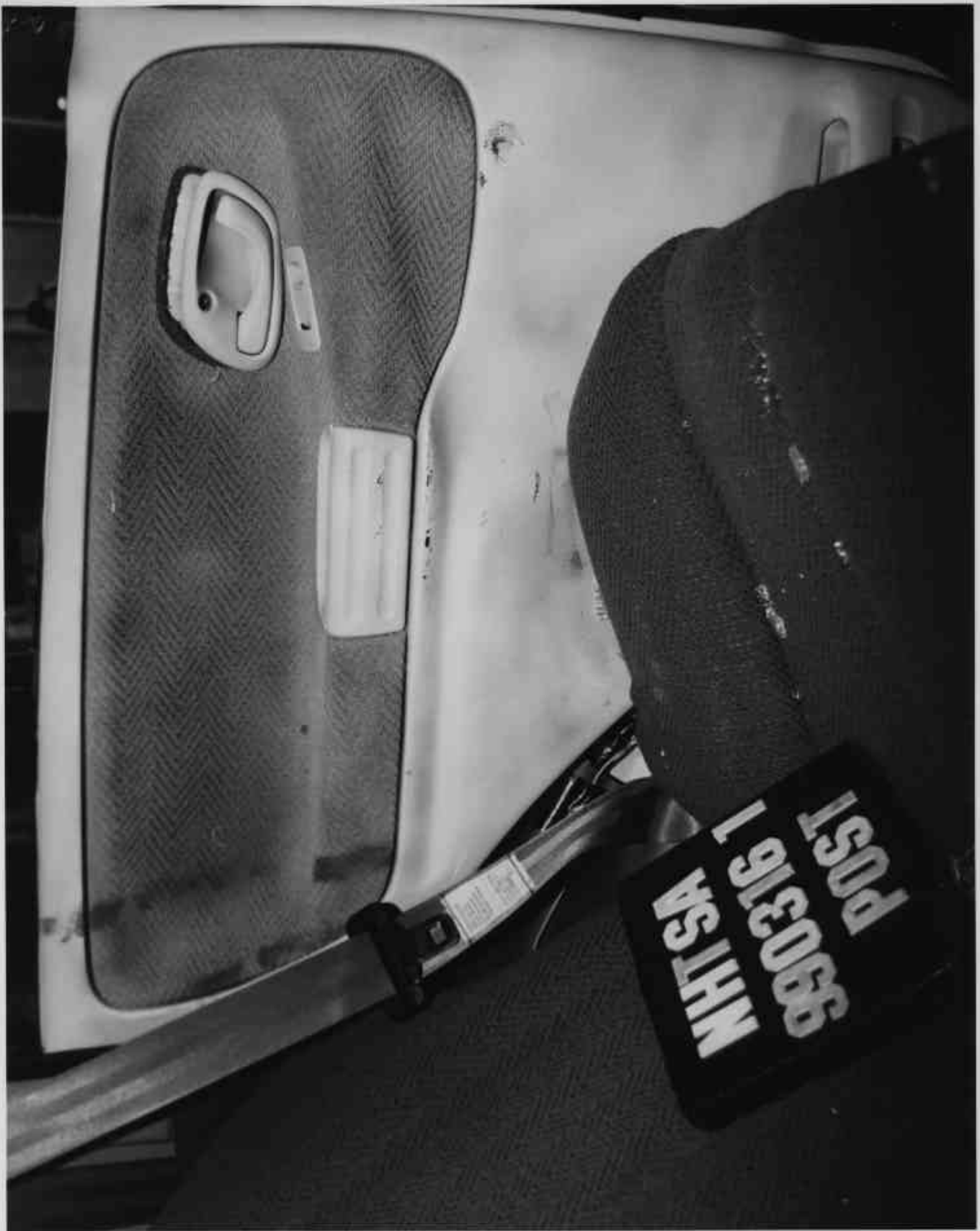
Figure A-45 Post-Test Interior of Rear Panel Showing SID Impact Locations A-48 990316
