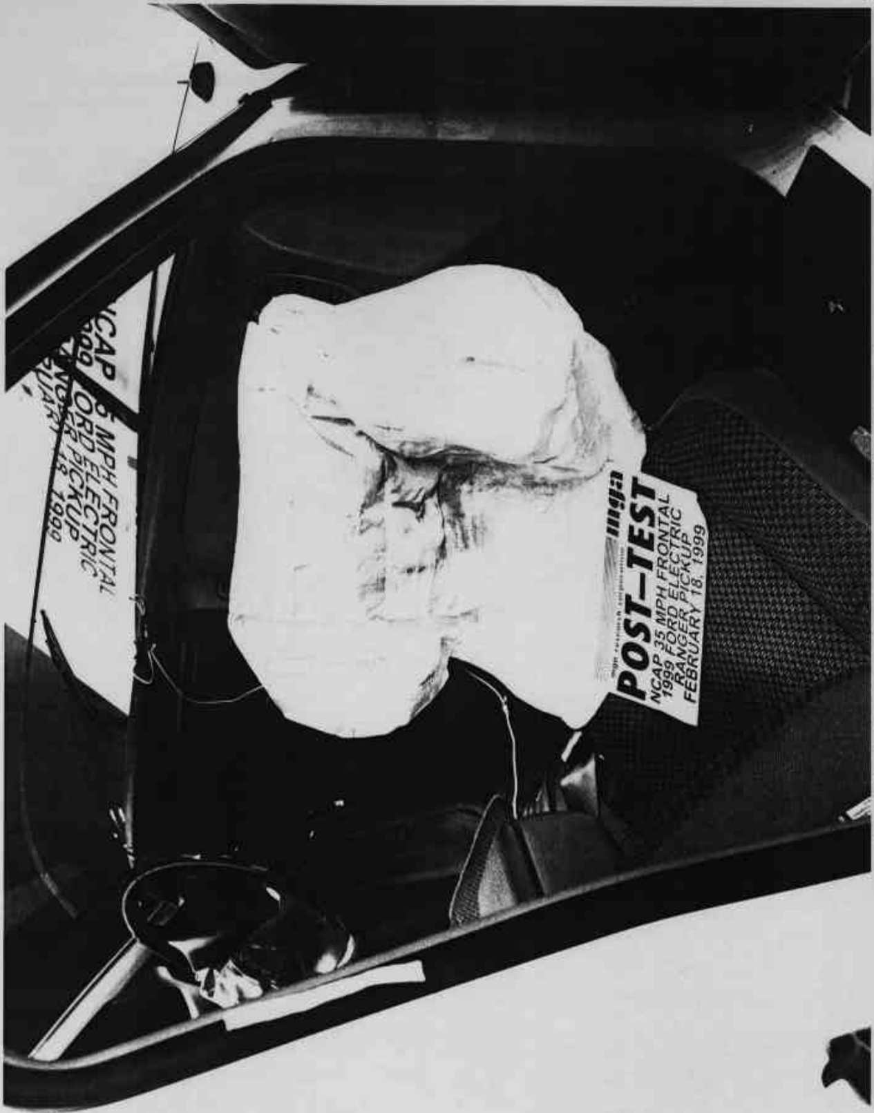
Photo No. A-39 - Post-Test Passenger Airbag Contact
