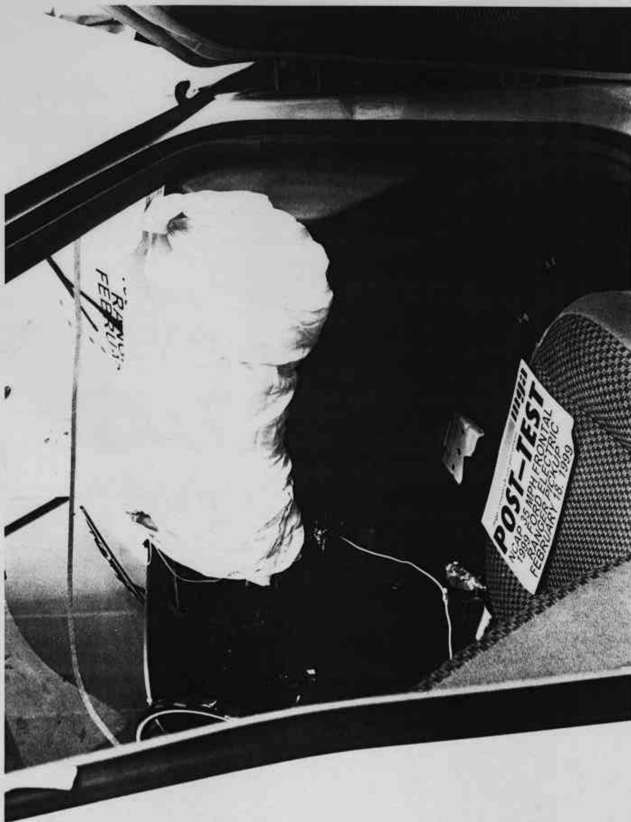
Photo No. A-40 - Post-Test Passenger Knee Contact View
