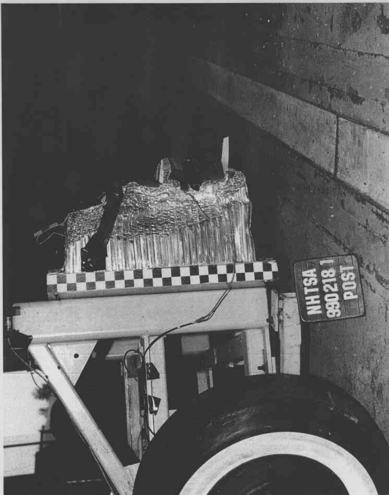
Figure A-16 Post-Test Right Side View of Impactor Face A-19
