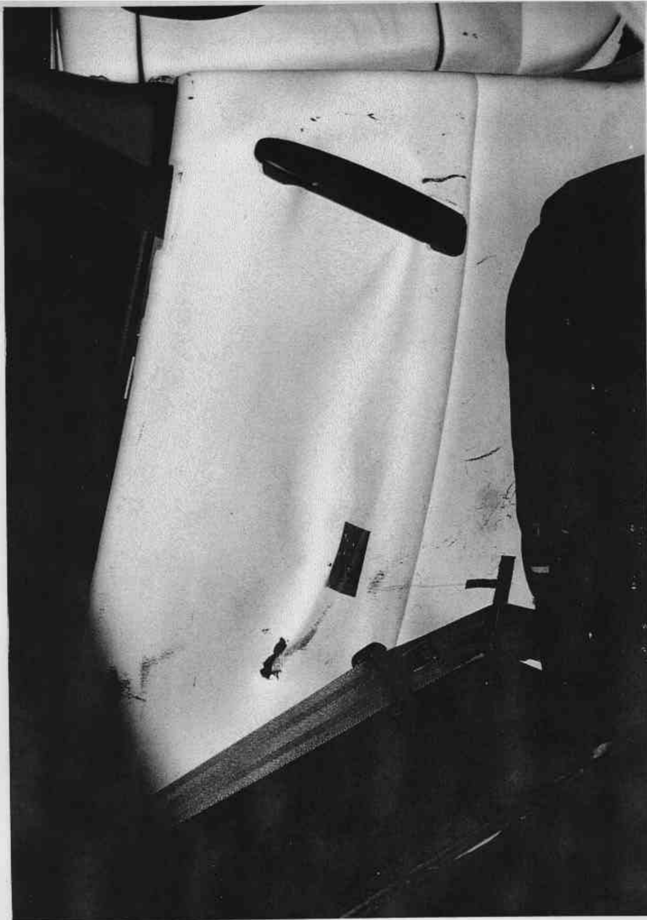
Figure A-28 POST-TEST REAR INTERIOR PANEL SHOWING SID IMPACT LOCATIONS
