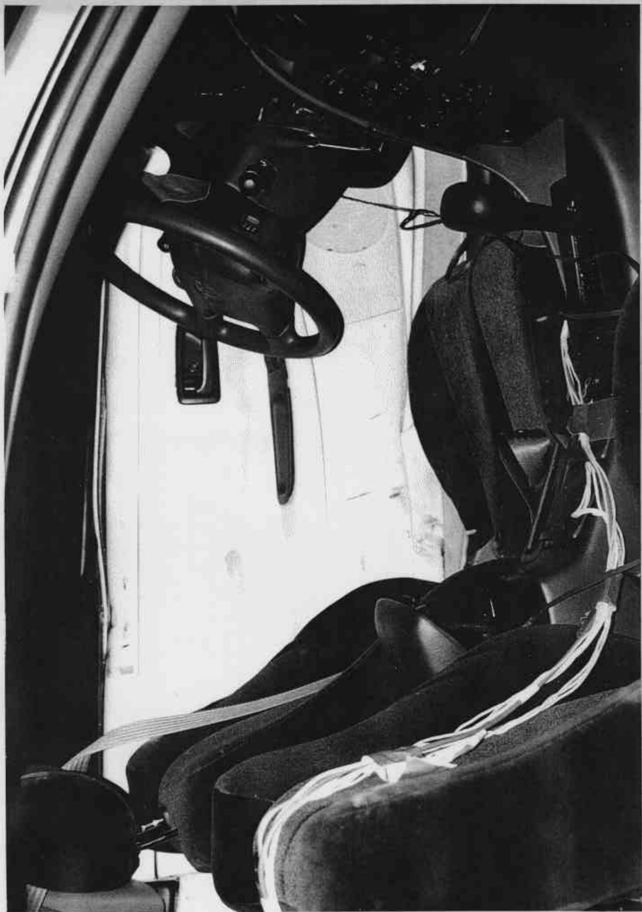
Figure A-26 POST-TEST INTERIOR OF FRONT DOOR SHOWING SID IMPACT LOCATIONS
