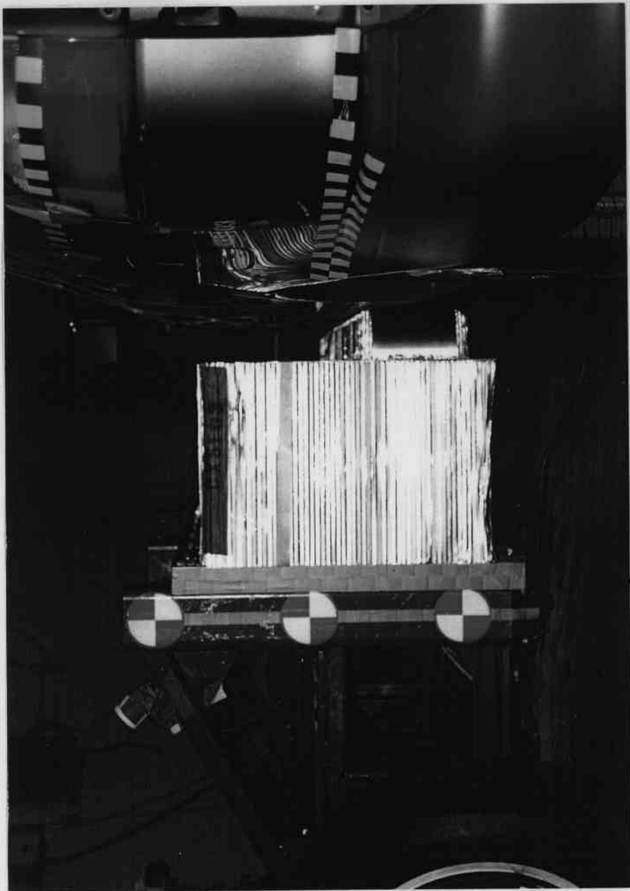
Figure A-30 PRE-TEST RIGHT SIDE VIEW OF MDB WITH IMPACTOR FACE IN POSITION
