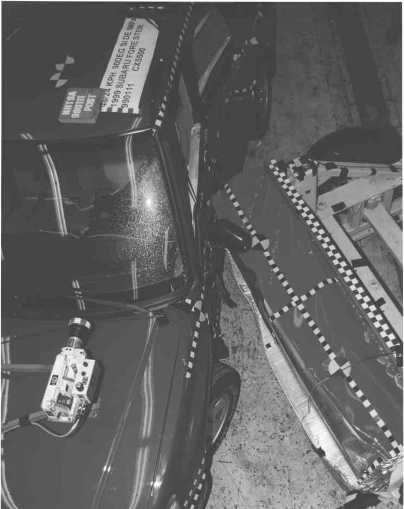
Figure A-16 Post-Test Overhead View of MDB Aligned with Vehicle
