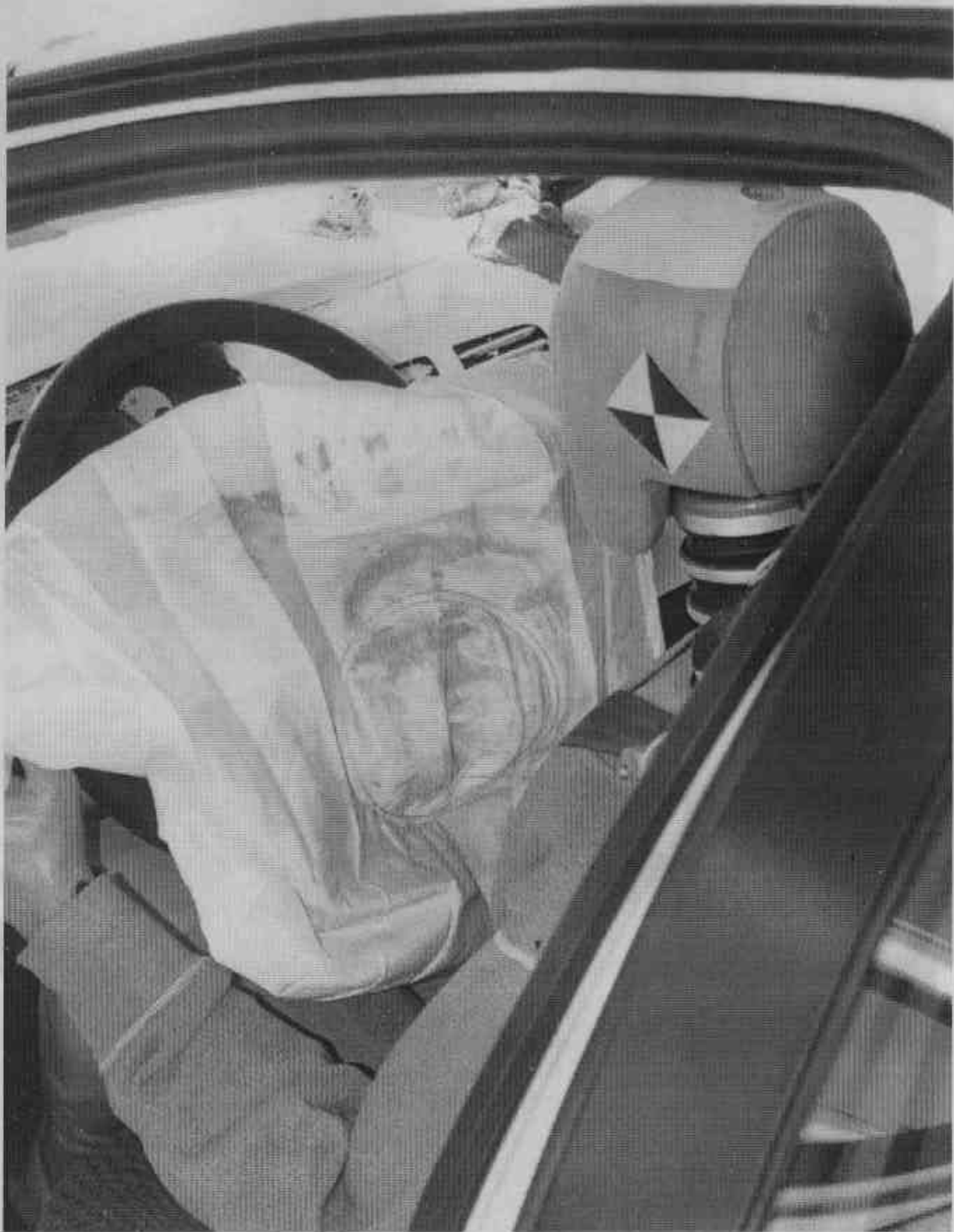
FIGURE A-40. POST TEST DRIVER DUMMY CONTACT
