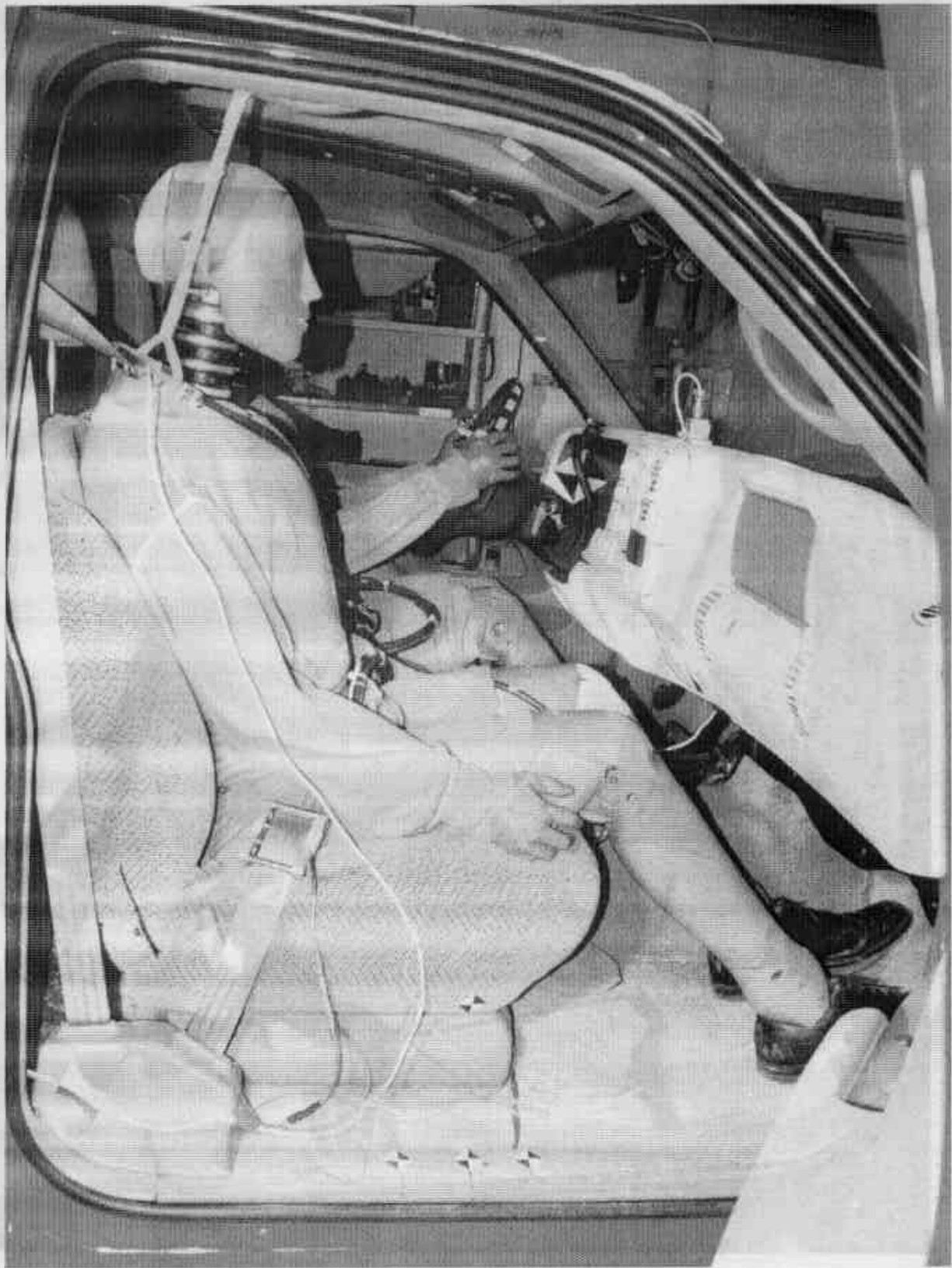
FIGURE A-47. PRETEST PASSENGER DUMMY (90° TO VEHICLE)
