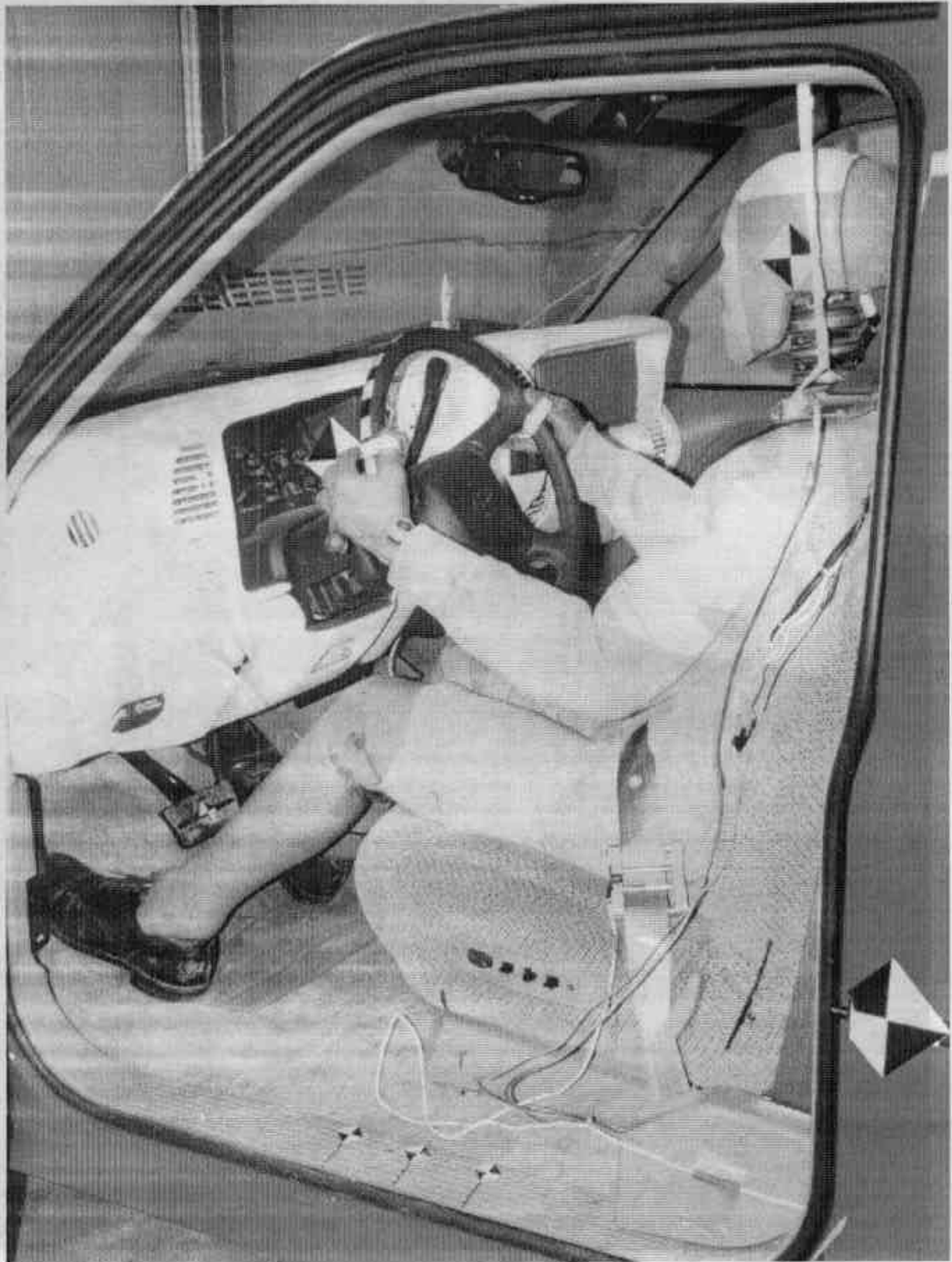
FIGURE A-29. PRETEST DRIVER DUMMY (DOOR OPEN)
