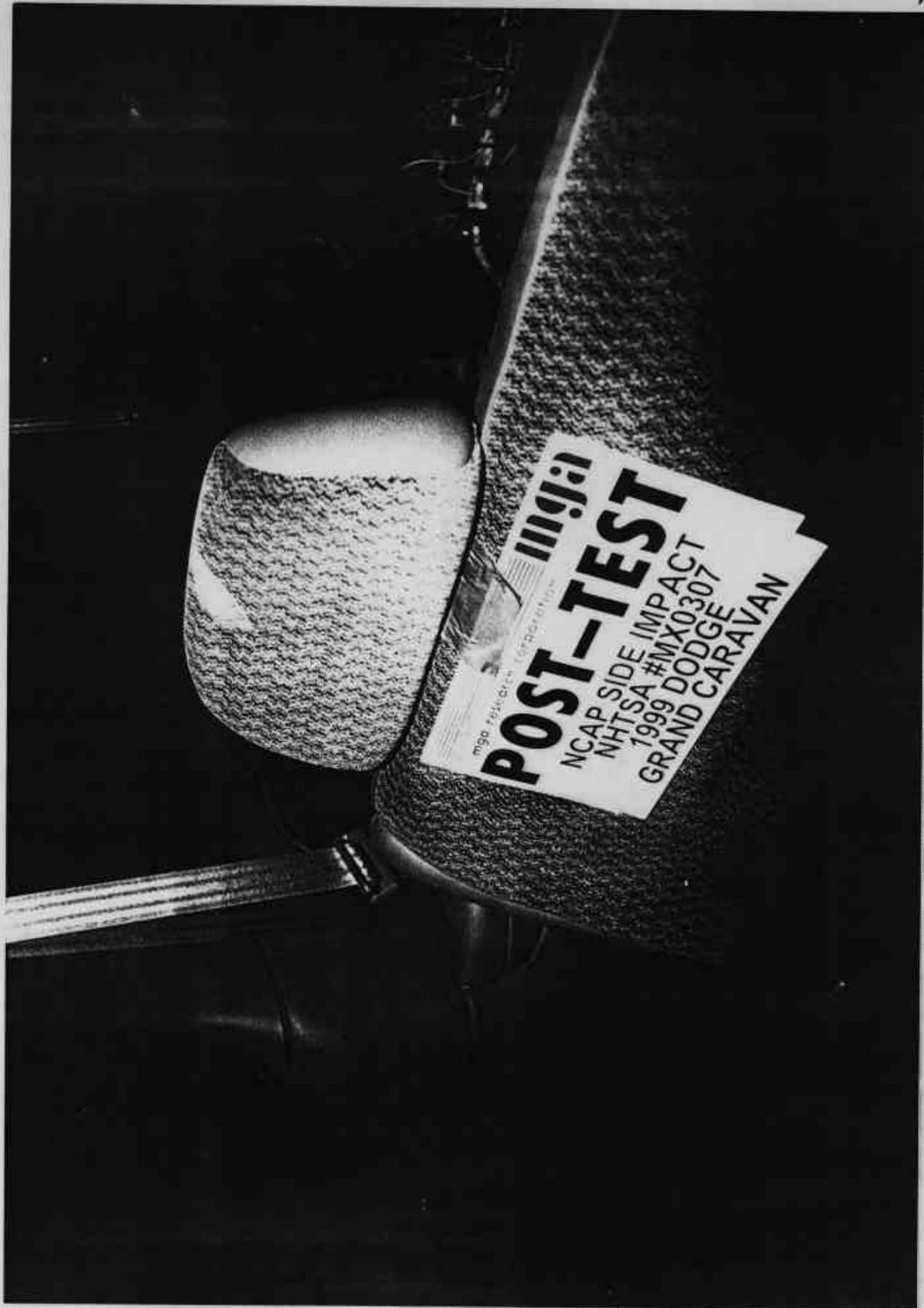
Photo No. A-39 - Post-Test Passenger Dummy Head Contact
