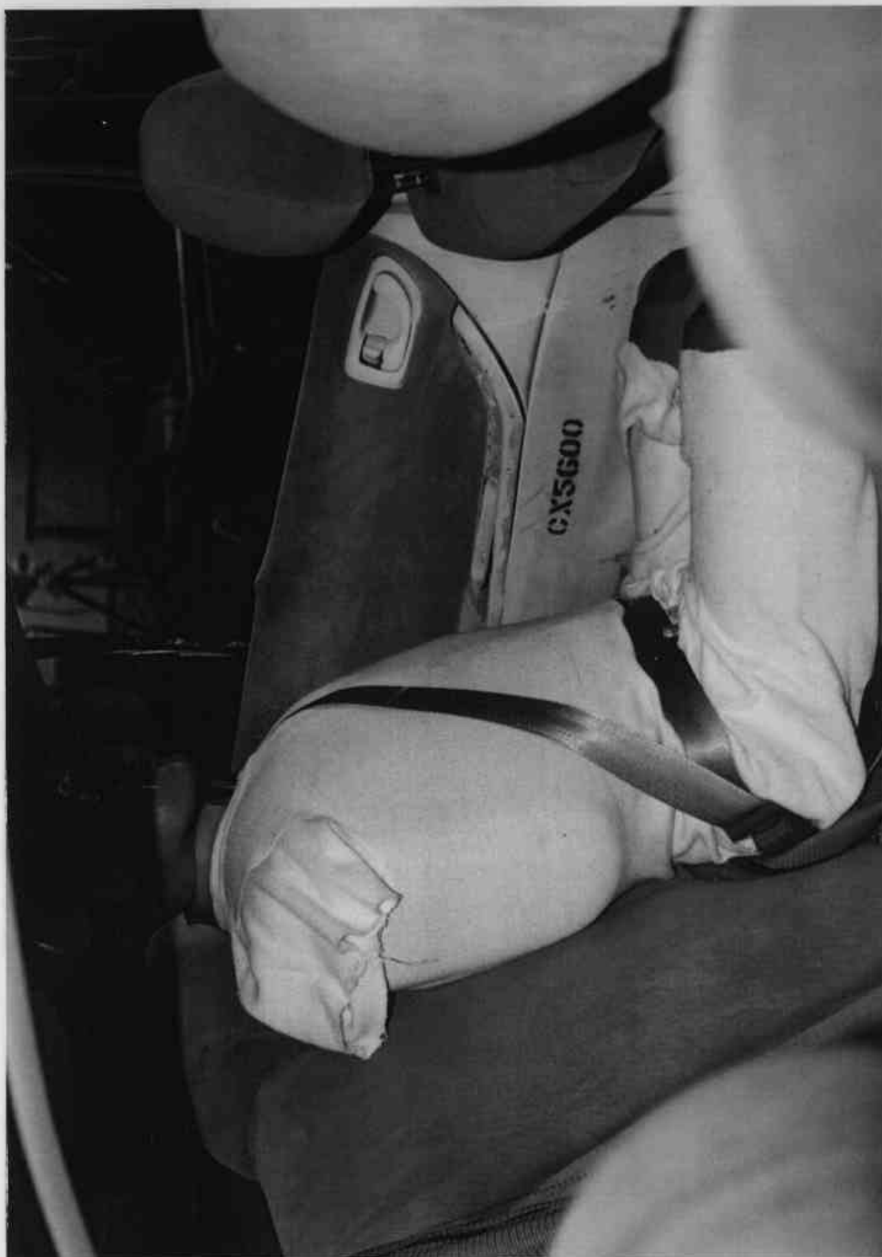
Figure A-20 POST-TEST RIGHT OCCUPANT COMPARTMENT VIEW OF REAR SID
